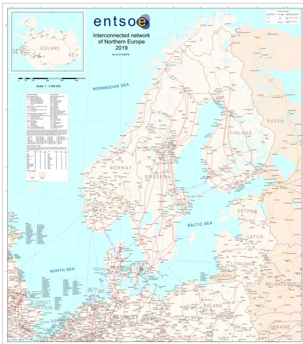
Figure 2-5: The power system in Northern Europe[1]
