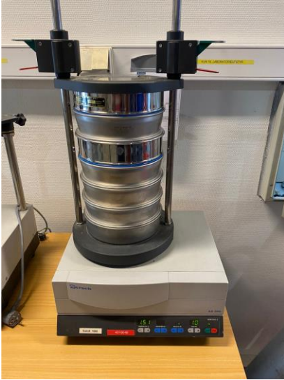
Figure 2.5: Determination of particle size distribution by sieving method.
