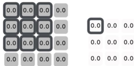
Figure 17: Example of how a 3x3 stride would down sample an image by removing the edge and top pixels in top left corner of the image.
