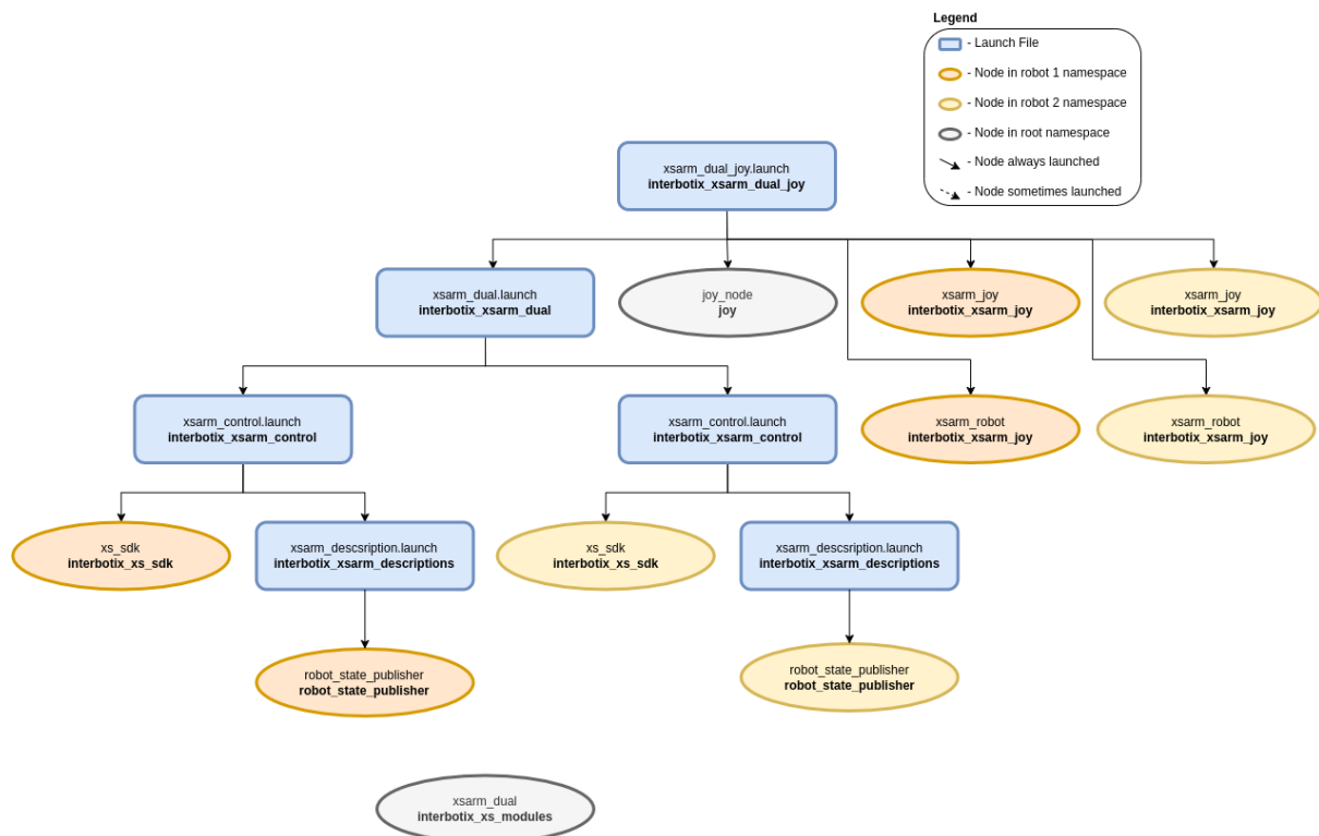
Figure 4.14: Dual Arm Joystick Control package structure [57]
