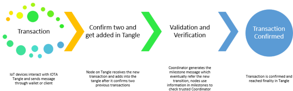
Figure 4: Transaction flow in IOTA Tangle
