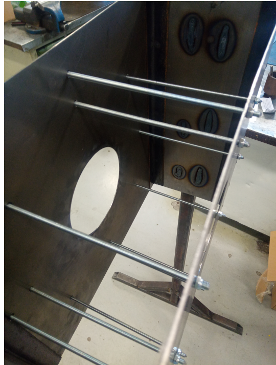
(b) The inside of the metal frame showing the thread rods.
