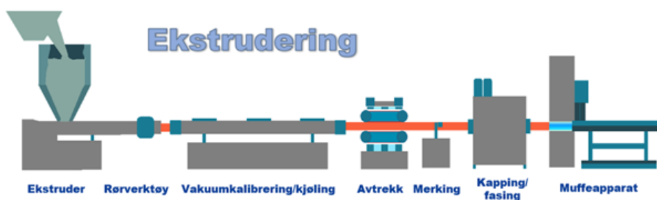
Figure 1.1: Simple figure of a extrusion line used to make plastic pipes.
