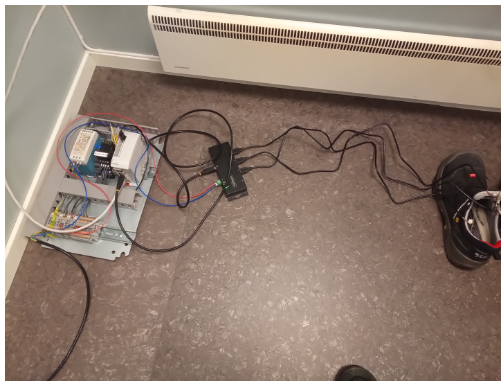
Figure 3.12: The setup of the test of the system being tested showing the plate from figure 3.8 with the power connected and the cameras connect through a USB hub.
