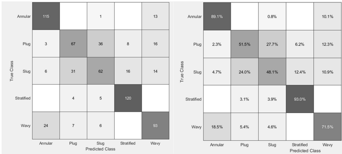
Figure 6.45: Confusion matrices of Ensemble learning algorithm for flow regime classification with US features as inputs and flow regimes as output
