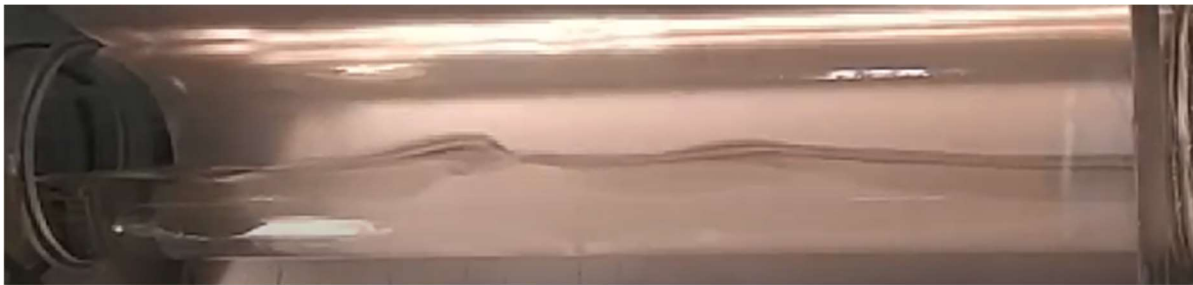
Figure 5.13: Wavy regime as seen in experiments
