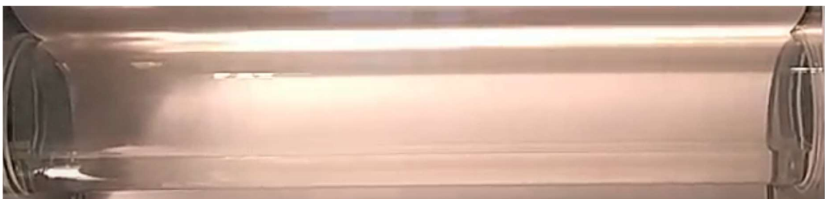
Figure 5.14: Stratified regime as seen in experiments
