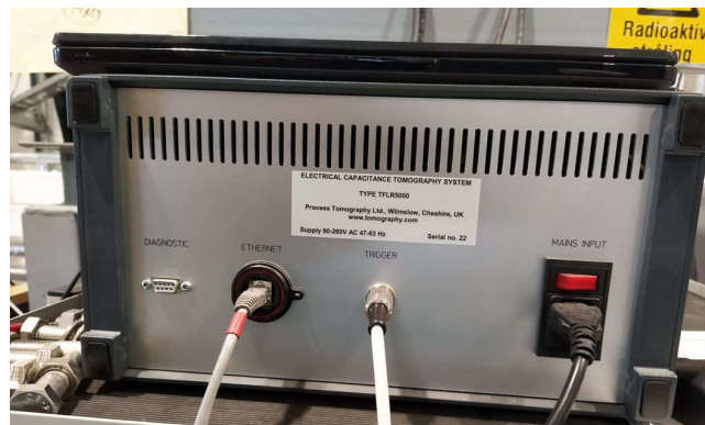
Figure 4.4: TFLR5000 ECT system control unit showing the communication and power ports
