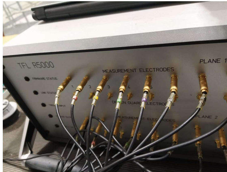
Figure 5.7: Connection of electrodes on 3 Feb 2023 with ECT 2-planes sensor
