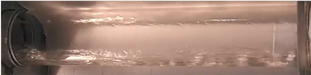
Figure 5.12: Annular regime as seen in experiments
