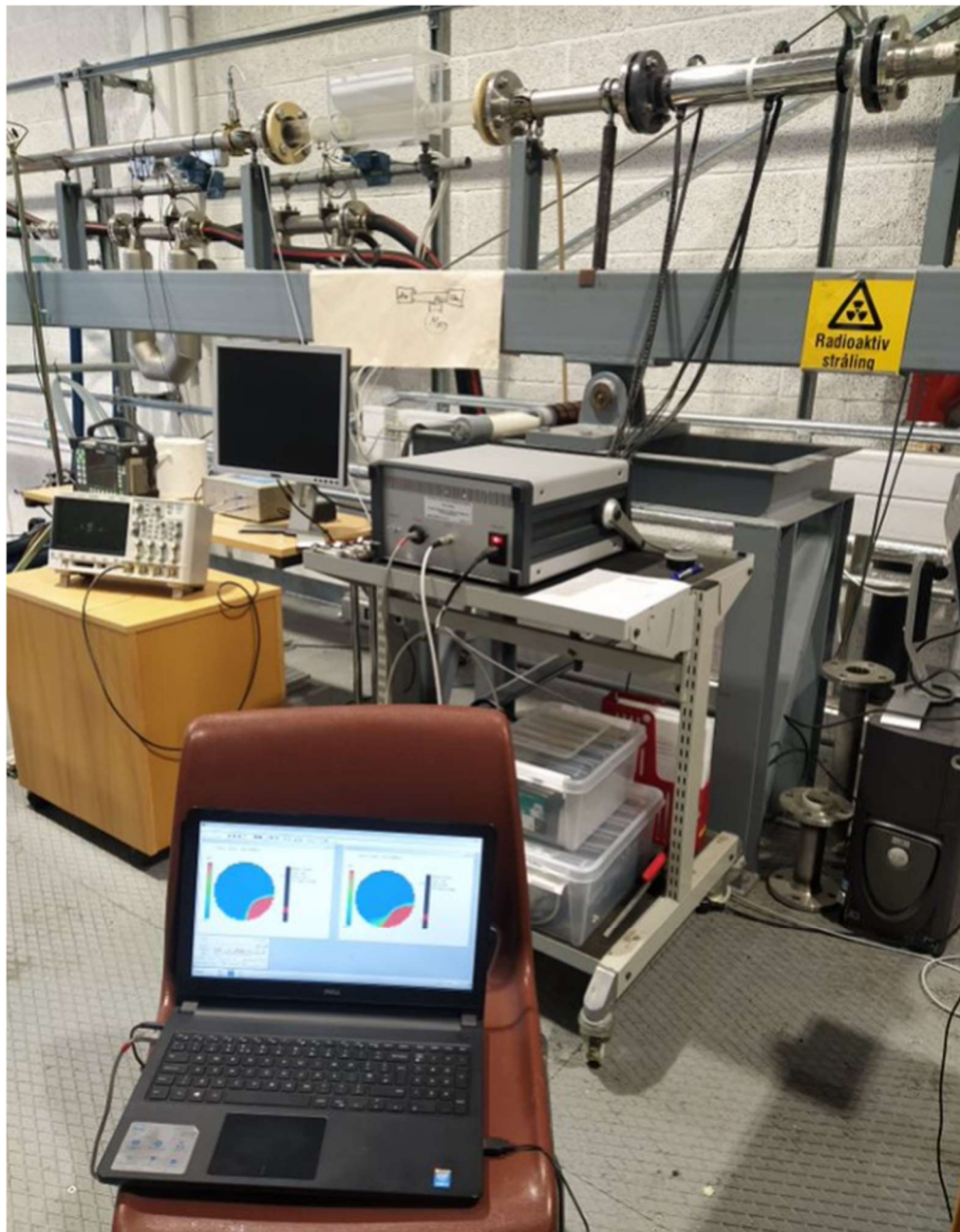
Figure 5.8: Ongoing ECT experiments on 3 Feb 2023 with 2-planes ECT sensor
