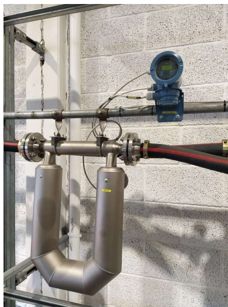
Figure 4.9: Coriolis meter FT115 for water installed at USN Rig
