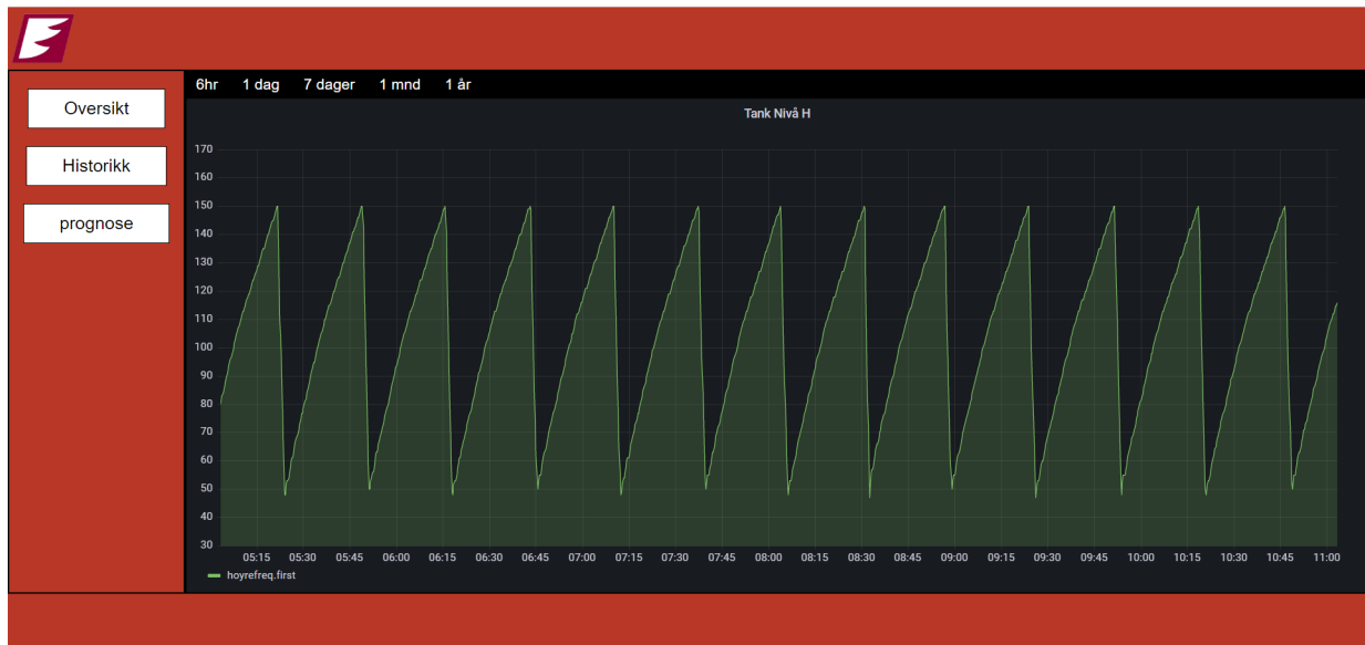
Figure 3.9: The inspect page of the HMI showing the historical data in detail.
