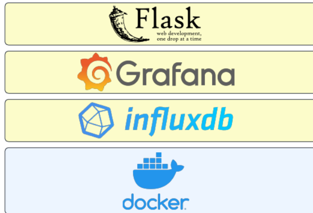
Figure 3.5: The Stack of the software architecture of the IoT system.
