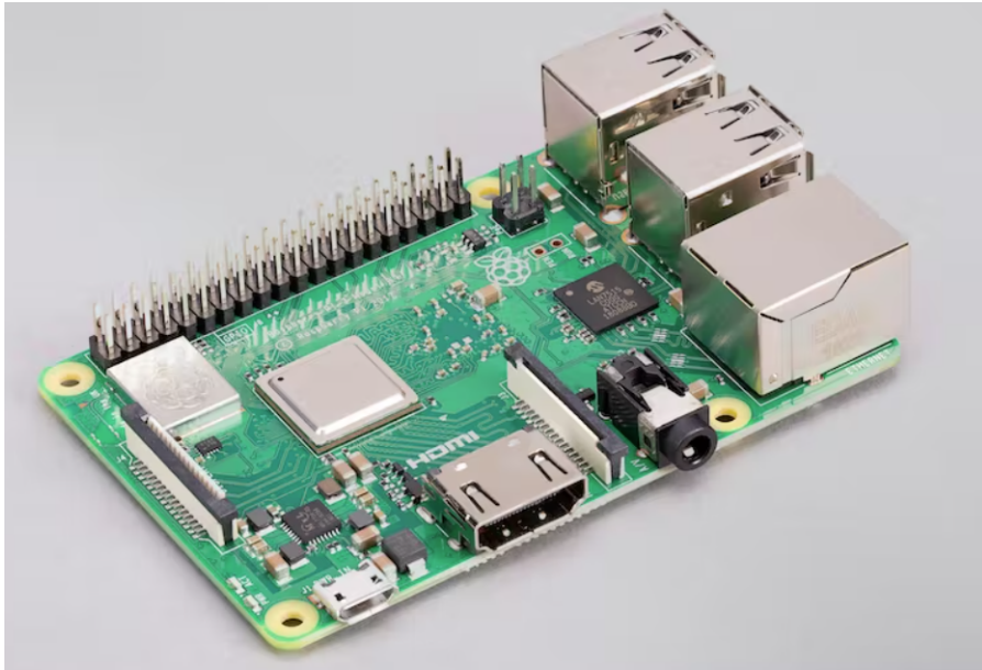
Figure 3.3: An image of the Raspberry Pi 3B+ taken from Raspberry Pi official website: RPI.com .
