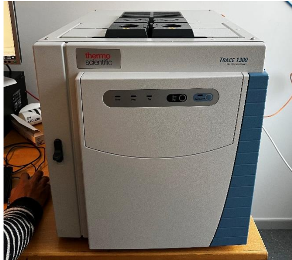
Fig 3-4 Trace 1300 gas chromatograph for gas analysis
