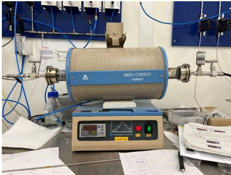
Fig 2-10 High temperature tube furnace
