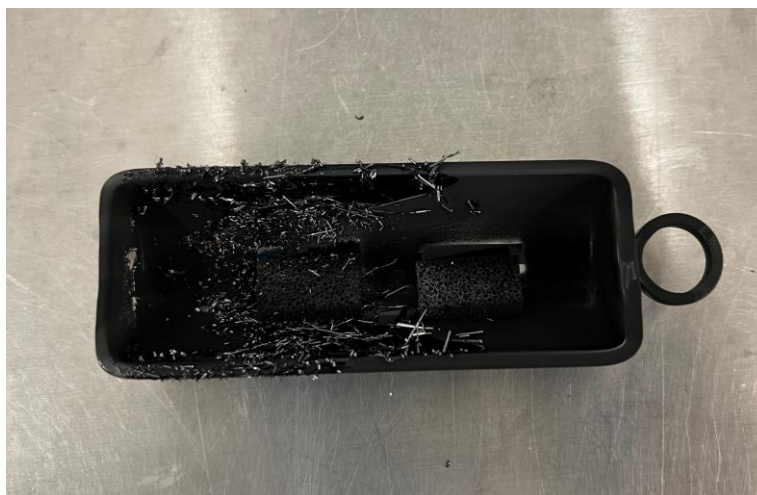
Fig 5-19 Black film formed on Quartz sample holder
