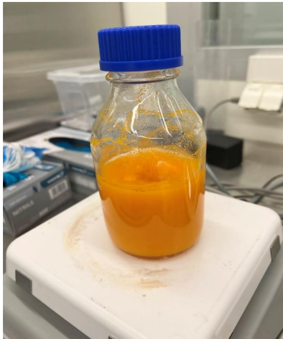
Fig 2-3 Ferrocene solution diluting by Magnetic Stirrer
