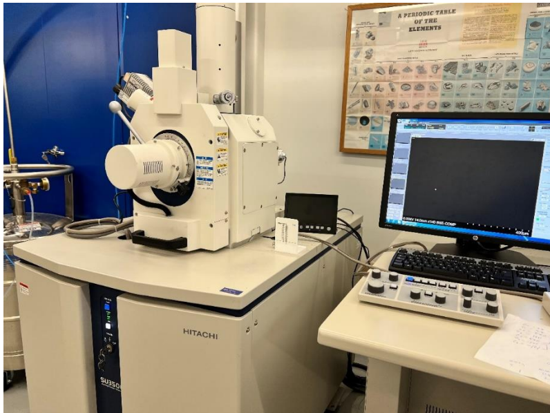
Fig 4-1 Hitachi SU3500 Scanning Electron Microscope
