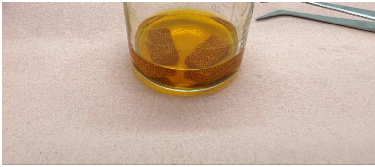
Fig 2-7 Copper foam dipped in ferrocene Solution
