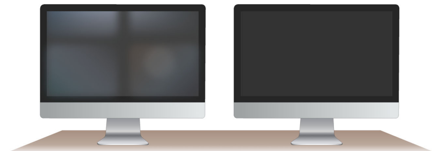
Fig. 5. Illustration of video display terminal (VDT) filter. Screen without VDT filter, illustrating glare (left). Screen with VDT filter, showing reduced glare (right). Copyright Sara T. Nøland.
