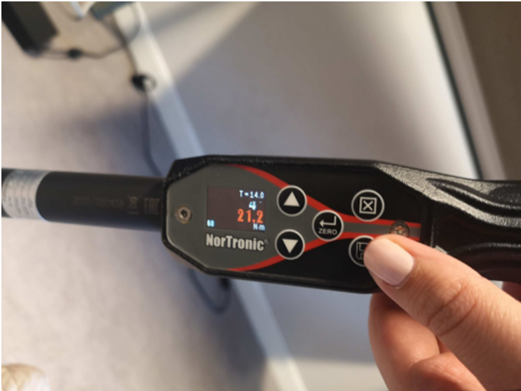
Figure 7: NorTronic torque wrench displaying a torque value torqued on a bolt
