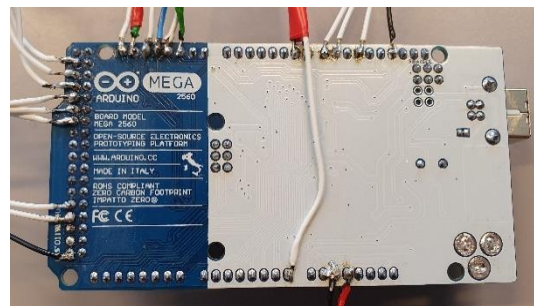
Figur 20: Loddingen under Arduino Mega.
