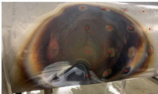
Fig. 6. Colour shift in the tank after the last test with sprinkler (test 4). Measuring locations highlighted with red.
