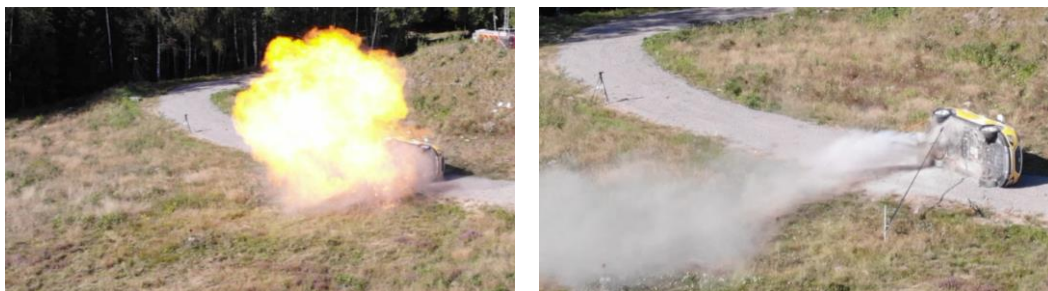
Fig. 5. The rupture of the small tank (left, test #1), and the puncture of the big tank (right, test #2). (Photo: Marcus Aronsson, SÄRF)
