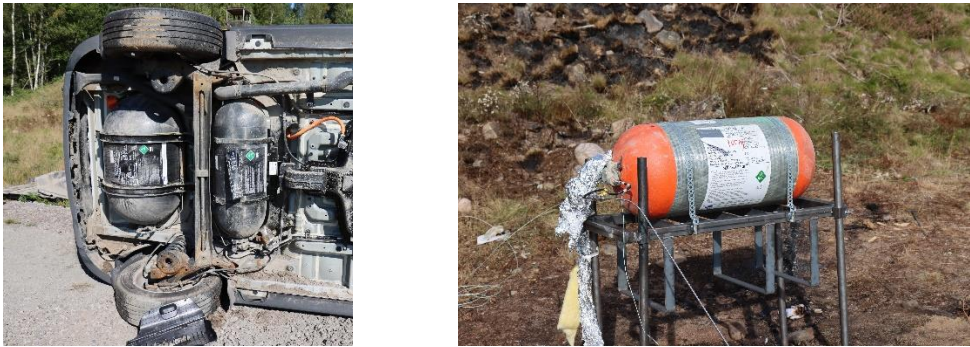
Fig. 2. The target: rear of the tilted hydrogen vehicle with the small and large tank (left) and a stand-alone tank (right) (Photo: RISE)
