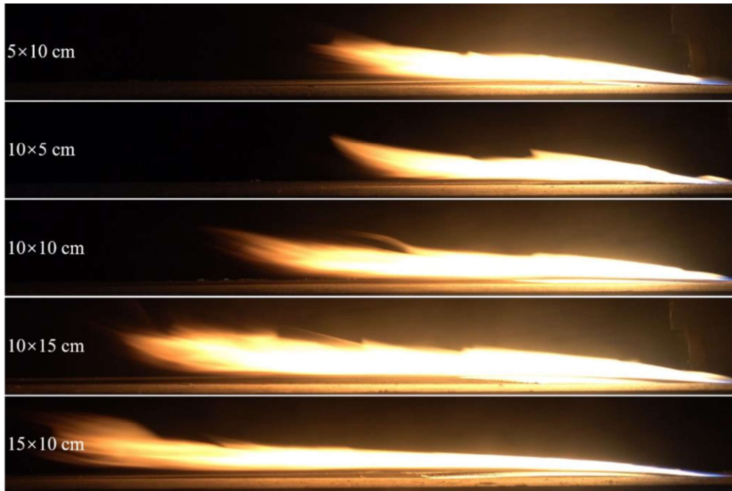
Fig.4. Image of stable combustion of PMMA plates with different sizes under forced flow
