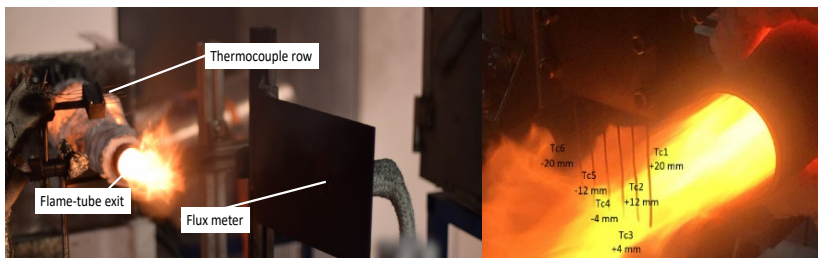
Fig. 6. View of the kerosene-burner test bench
