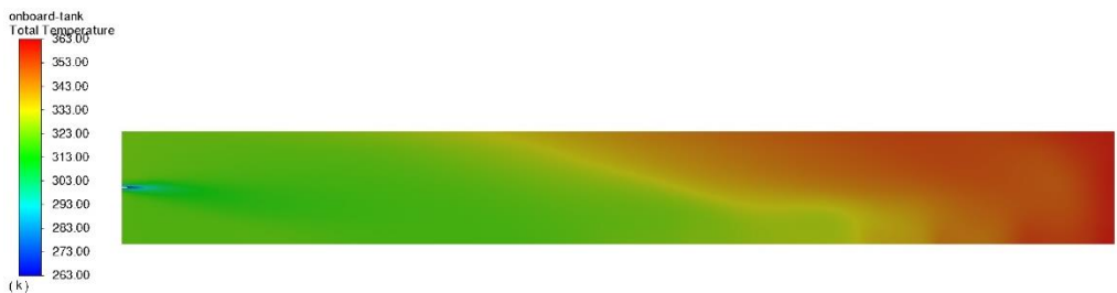
Figure 5 - Capability of temperature non-uniformity prediction in the CFD model.
