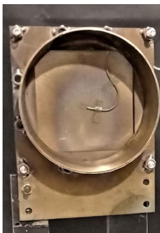
Fig 3. Steel plate with the thermocouple welded on it
