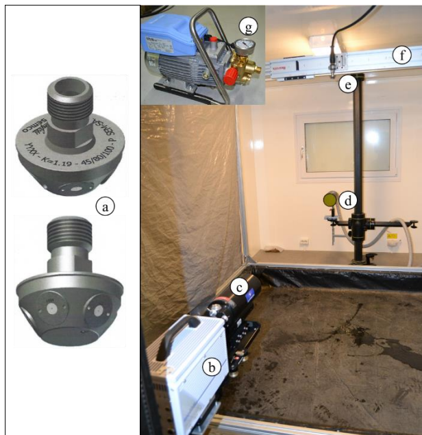
Fig. 2. Experimental setup with a) Danfoss mist nozzle [14], b) high-speed camera, c) microscope lens, d) laser front optics, e) mist nozzle with mount, f) traverse, g) Kränzle HD 10/122 TS high-pressure washer pump.
