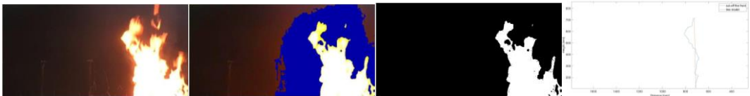
Fig. 4. Flame front identification steps (from left to right): Cropped image, “chromatically” processed image, binary black-and-white image, flame front identification.
