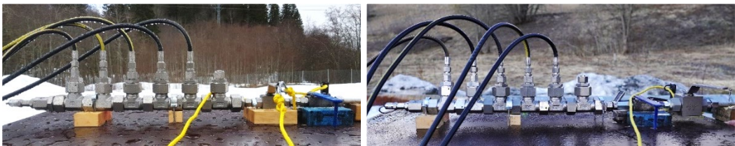
Fig. 3. Hydrogen manifold. From left to right are the pressure transducer, 5 hoses from hydrogen bottles, ball valve remotely operated by yellow ropes (left figure)/Coriolis mass flow meter (right figure), Coriolis mass flow meter (left figure)/ball valve remotely operated by yellow ropes (right figure), and the pipe leading to the jet nozzle.
