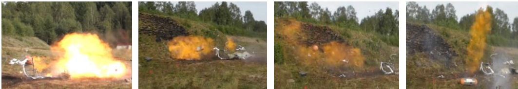
Fig. 8. A sequence of pictures showing the penetration on the first shot in #5b, from left to right.
