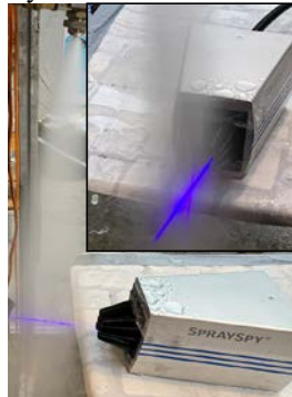
Fig. 3. Characterization of the SU42 spray with the SpraySpy system.
