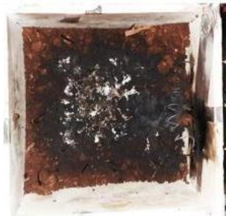
Fig. 12. Smoldering residue seen inside the Reactor
