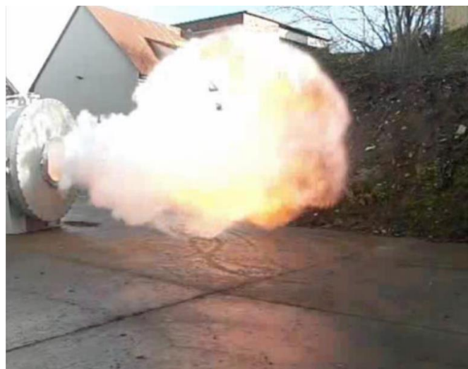
Fig. 2. A snapshot of the vented corn starch dust explosion in the 11.5 m 3 vessel with a circular vent opening.
