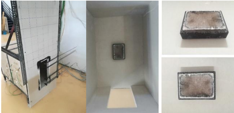
Fig. 1. Fire compartment (left) and porous burner (right).
