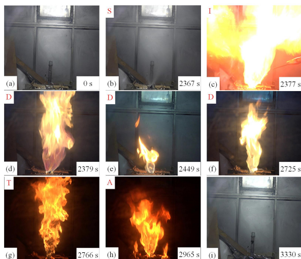
Fig. 3. Thermal runaway process of the LIB without extinguishing agents
