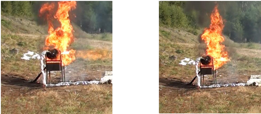
Fig. 7. A small jet flame following the penetration on the first shot in 4a (left) and 4b (right). (Photo: RISE)
