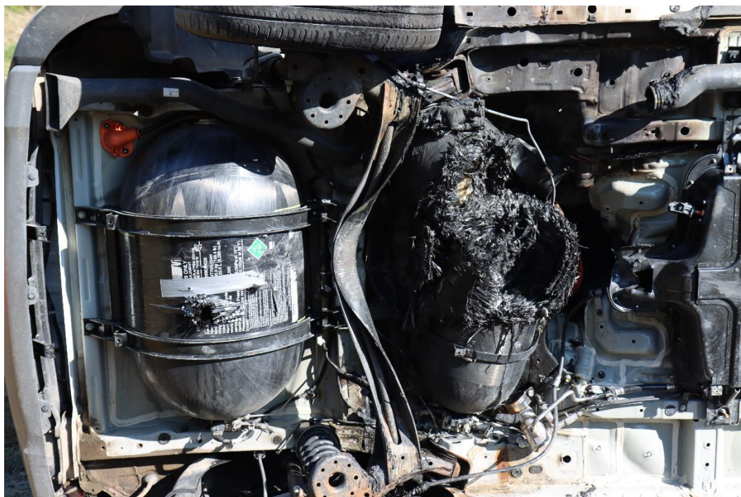
Fig. 6. Punctured big tank (left, test #2) and ruptured small tank (right, test #1). (Photo: RISE)
