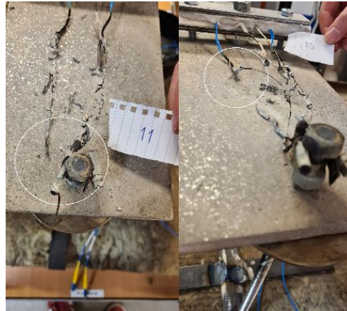
Fig. 5. Cables post-test with the breaking points highlighted [4].
