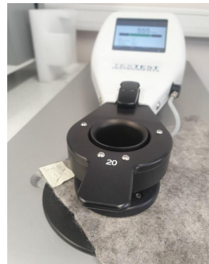
Fig.20 - Air permeability test
