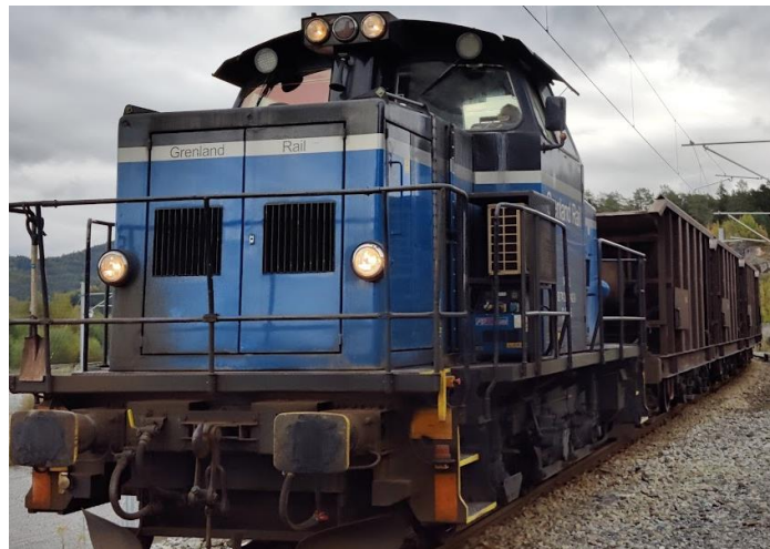
Figure 1.1 Subject vehicle, a 1972 Skd 226, weighing 32tonnes (without carriages)
