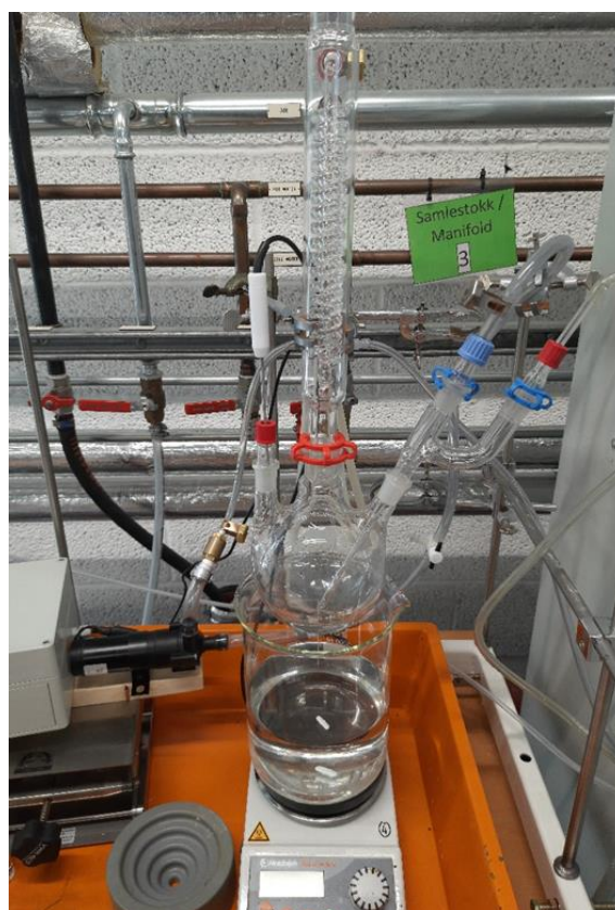
Figure 4.3: Three neck glass reactor.
