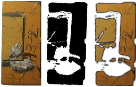
Figure 7 – Crack formations in a SLID transducer. Top-view photography of the sample (left image), SAM-image of the same sample (middle image), and the SAM-image overlaid the photography (right image).
