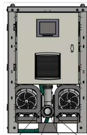
Figure 2.10: Control cabinet placement on the NOMAD vacuum unit, as shown in the general arrangement (GA) drawing [2]
