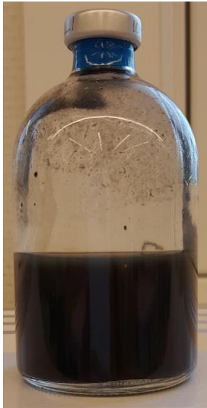
Figure 3.7: Serum bottle as a bioreactor.
