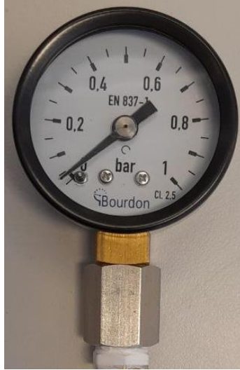
Figure 3.9: Bourdon Dial Pressure Gauge 1bar, MAT1D10B15.
