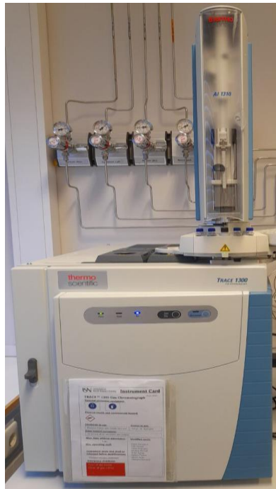
Figure 3.8: THERMO Scientific TRACE™ 1300 Gas Chromatograph.
