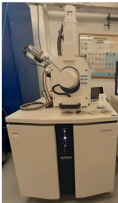
Figure 3.4: Hitachi SU3500 Scanning Electron Microscopy.
