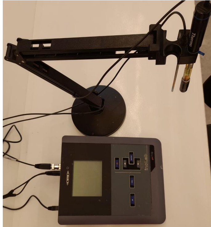
Figure 3.10: pH meter WTW inoLab 7110.
