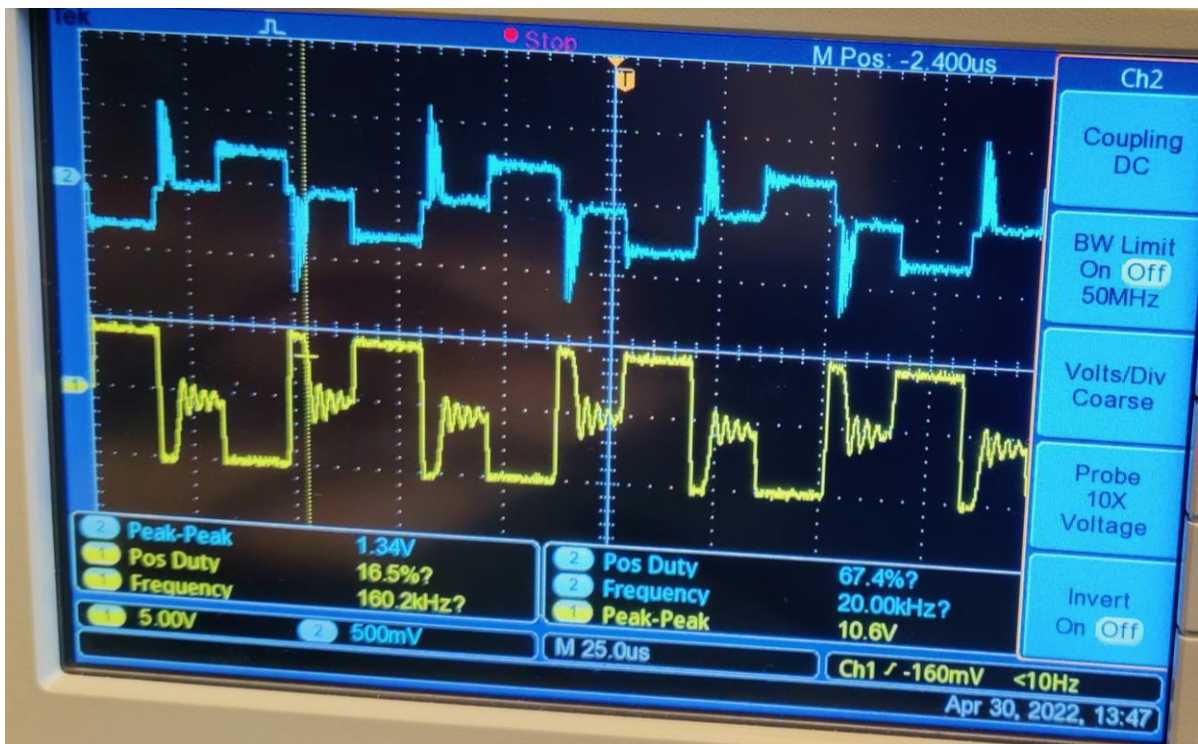
Figure 5-5 Waveforms on the primary (yellow) and the secondary side (blue) of the transformer with 50% duty cycle
