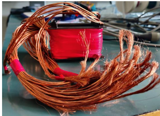
Figure 4-13 Transformer windings with the Litz wire
