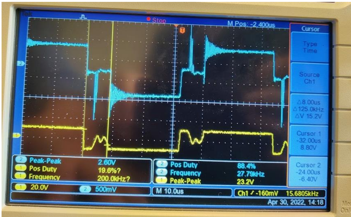
Figure 5-6 Waveforms on the primary (yellow) and the secondary side (blue) of the transformer with 75% duty cycle
