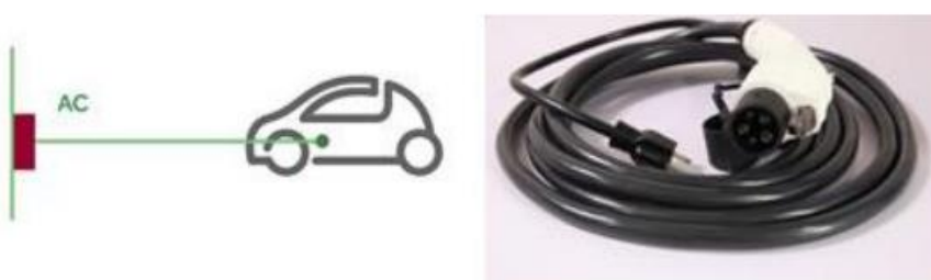
Figure 3-5:EV charging Mode 1 and cable[19]
