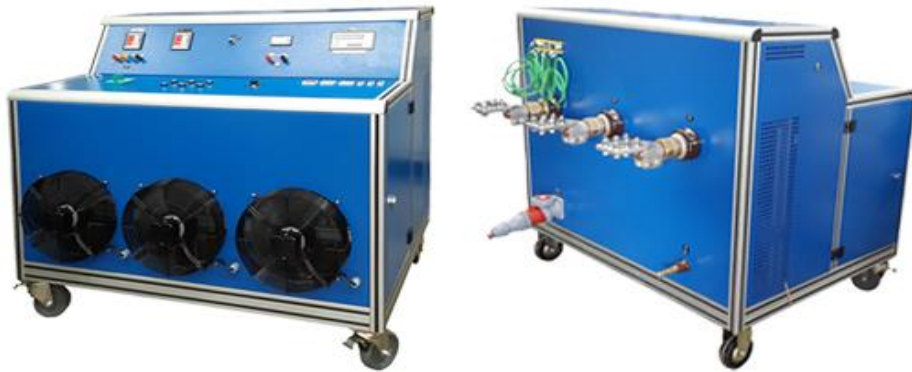
Figure 6-3:Current injection tester[44]
