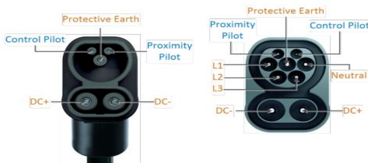
Figure 6-12: CCS2 inlet and connector with pin descriptions[45]
