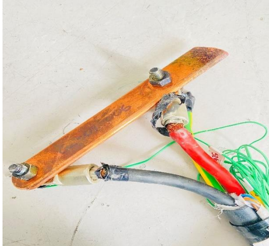
Figure 6-13:Short circuit at the end of connector
