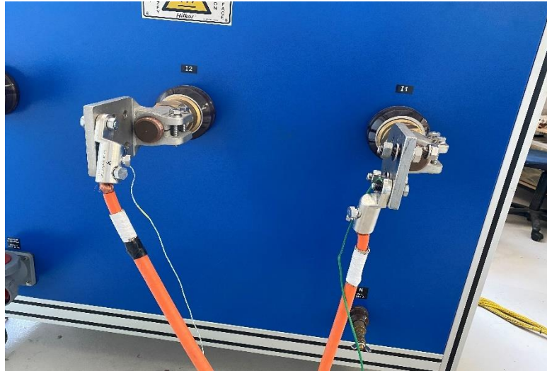
Figure 6-15: Inlet connection with power supply
