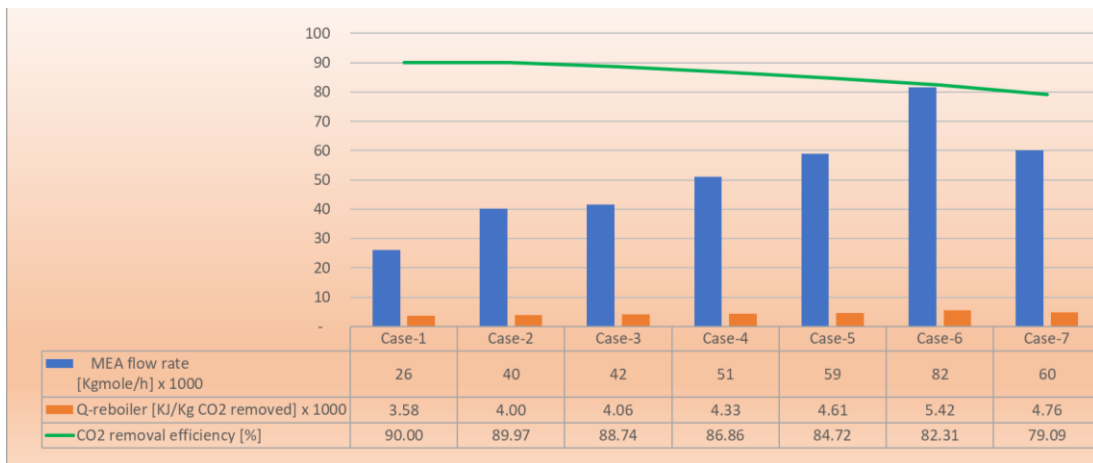
Figure 8.4: CO 2 removal efficiency, energy and MEA demand dependency on number of packing stages in the absorber column.
