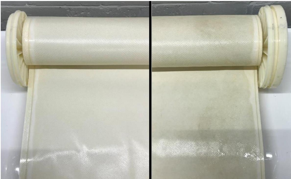
Figure 2.11: Fouling on a lead element in the 1<sup>st</sup> stage of SRU B. Concentrate side to the left and feed side to the right. Fouling is mainly biofouling and is most evident on feed side. Membrane autopsy performed by Avista.
