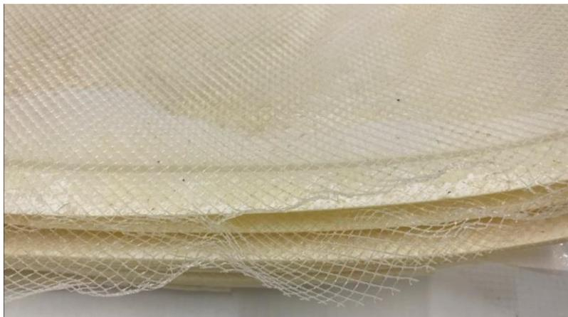
Figure 2.13: Damaged spacer due to telescoping in one of the lead elements in the 1<sup>st</sup> stage of SRU B. Membrane autopsy performed by Avista.
