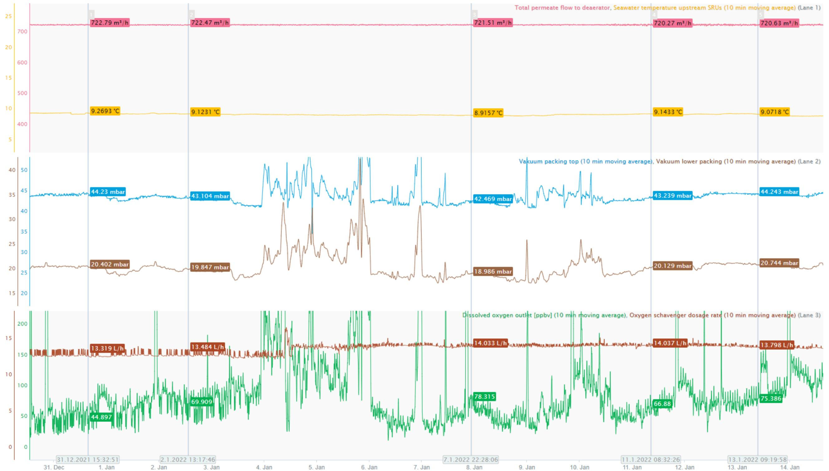
Figure 5.22: Deaerator parameters during normal operation at a seawater production and temperature of ~720 m<sup>3</sup>/h and 9.1 °C. The upper lane shows the seawater temperature and flow entering the deaerator. The middle lane presents the deaerator stage pressures where the top packing is the 1<sup>st</sup> stage while the lower packing is the 2<sup>nd</sup> stage. The lower lane shows the dissolved oxygen and oxygen scavenger dosage rate.
