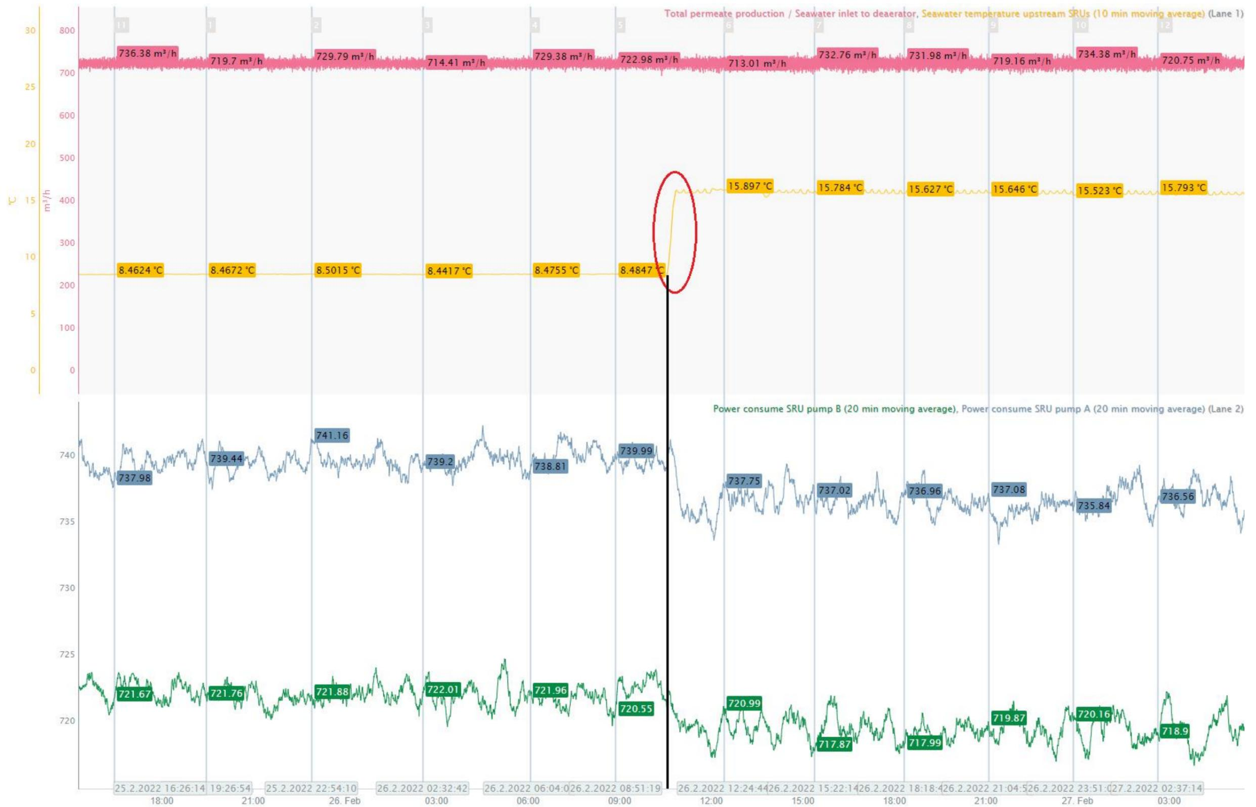
Figure 5.12: Power consumption [kW] for the SRU pumps upstream the SRUs correlated to the increased seawater temperature upon initiation of Test 1 marked with the red circle. The upper lane shows total permeate production and seawater temperature upstream the ultrafiltration. The lower lane shows the SRU pumps power consumption in kW.
