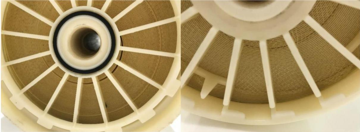
Figure 2.12: Telescoping of feed spacer on a lead element in the 1<sup>st</sup> stage of SRU B. Gapping in the membrane feed side to the left. And telescoped feed spacer at the concentrate side to the right. Membrane autopsy performed by Avista.
