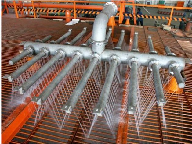
Figure 2.16: Pipe liquid distributor tested with liquid. [11]
