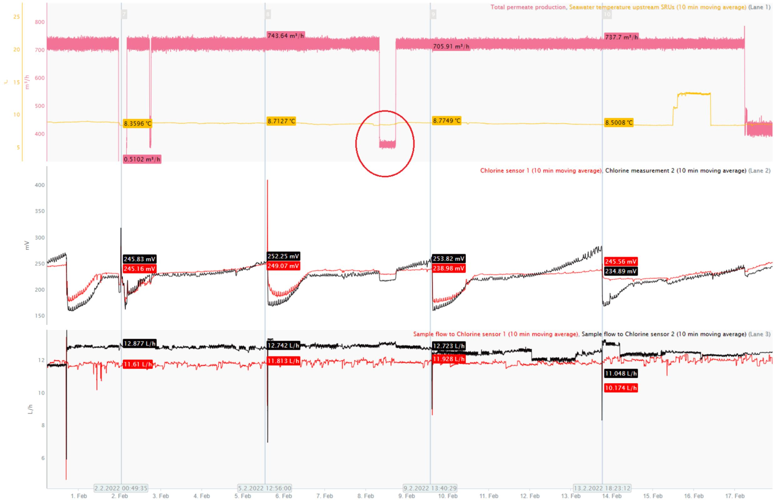
Figure 5.14: Flushing frequency during normal operation when ~8.5 °C seawater temperature and 720 m³/h permeate production. The upper lane shows total permeate production and seawater temperature. The middle and lower lane shows chlorine measurements (in mV) and sample flowrate to the sensors. The red circle indicates a change in total permeate production which excludes that particular flushing time interval from the assessment.
