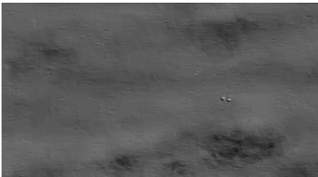
FIGURE 1.1: Feature map created by convolving an image with weights extracted from the modified ResNet used in this thesis. The two dots in the right part of the image are heat signatures, also known as IR small targets.
