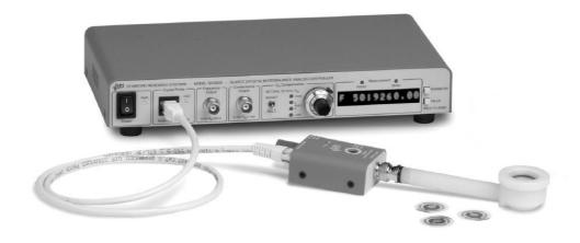
Figure 7: Complete QCM setup consisting of QCM200 digital controller, QCM25 crystal oscillator, crystal holder, and three quartz crystal sensors
