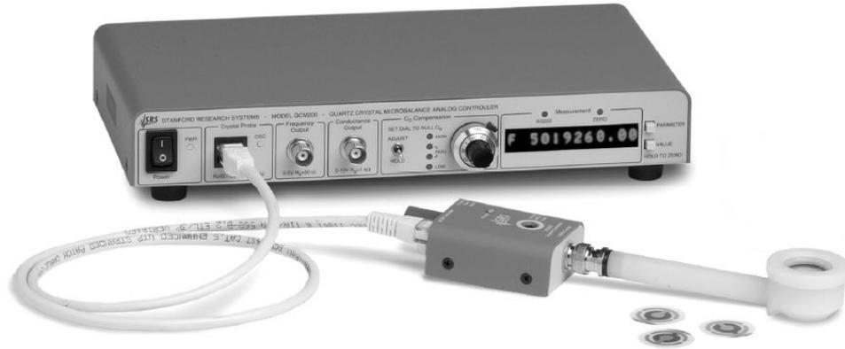
Figure 7: Complete QCM setup consisting of QCM200 digital controller, QCM25 crystal oscillator, crystal holder, and three quartz crystal sensors
