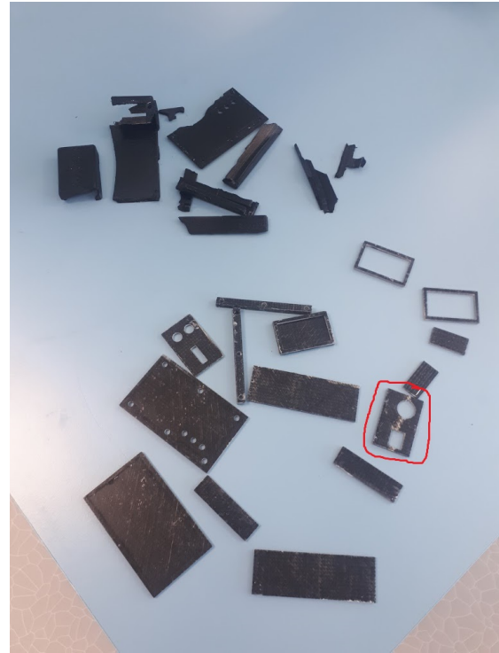
Figure 48: PETG- and nano casing after test
