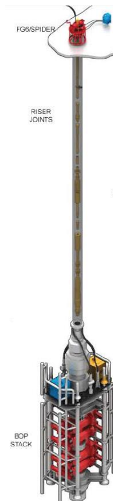
Figure 3: Marine riser and BOP
