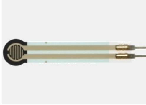
Figure 13: Small force sensing resistor.
