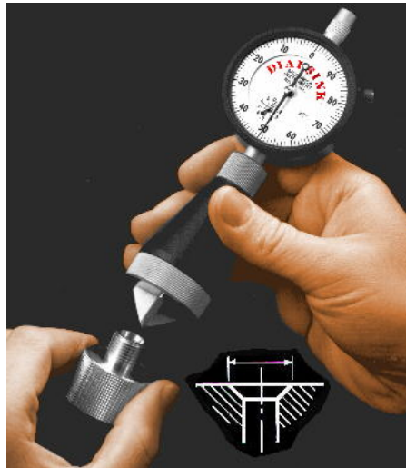
Figure 28: Countersink gauge example.
