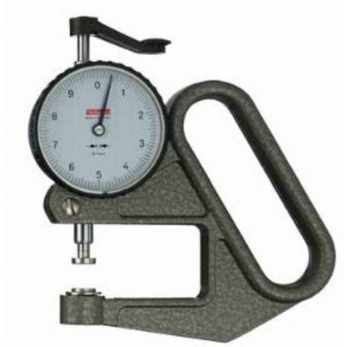
Figure 26: Example of mechanical thickness gauge.
