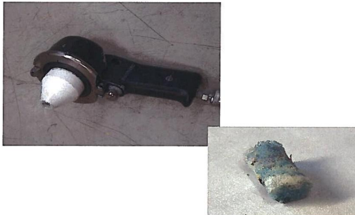
Figure 4: Jet cleaner with soft plug
