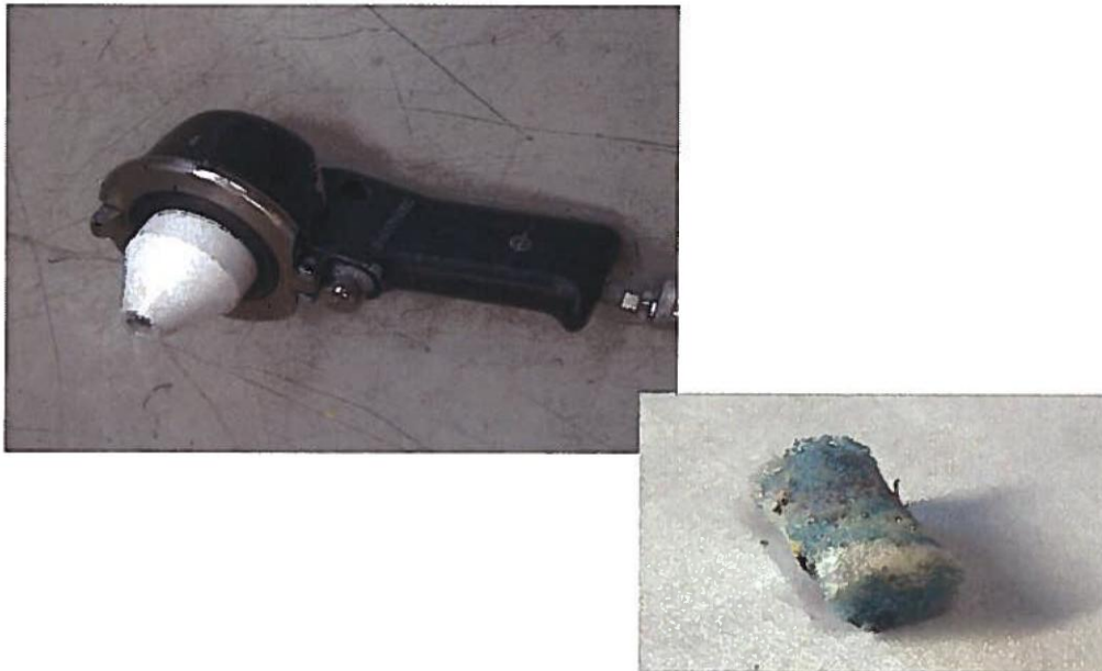
Figure 4: Jet cleaner with soft plug
