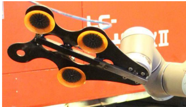
Figure 132: Vacuum gripper tool, 3 cups
