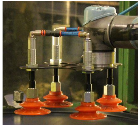
Figure 131: Vacuum gripper tool, 4 cups
