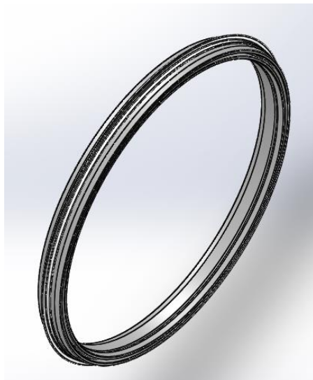
Figure 1: Rubber ring mounted around the seal ring (lhs)
