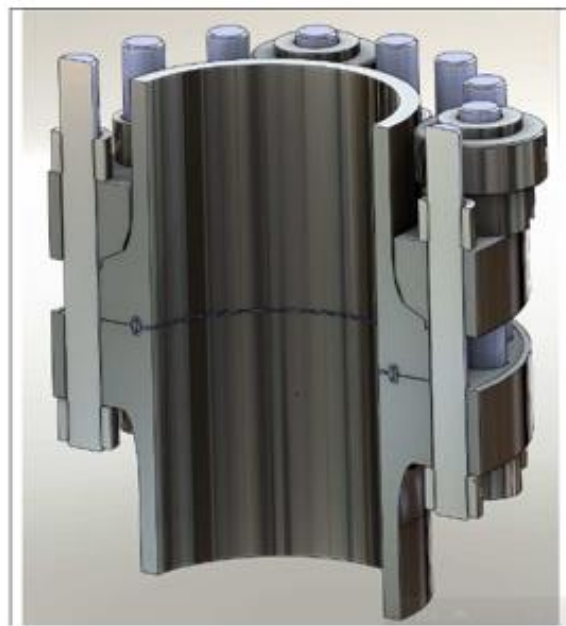
Figure 19: Swivel flange [7]
