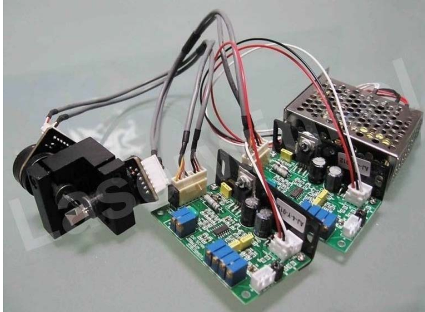
Figure 17: Physical galvanometer setup [22]
