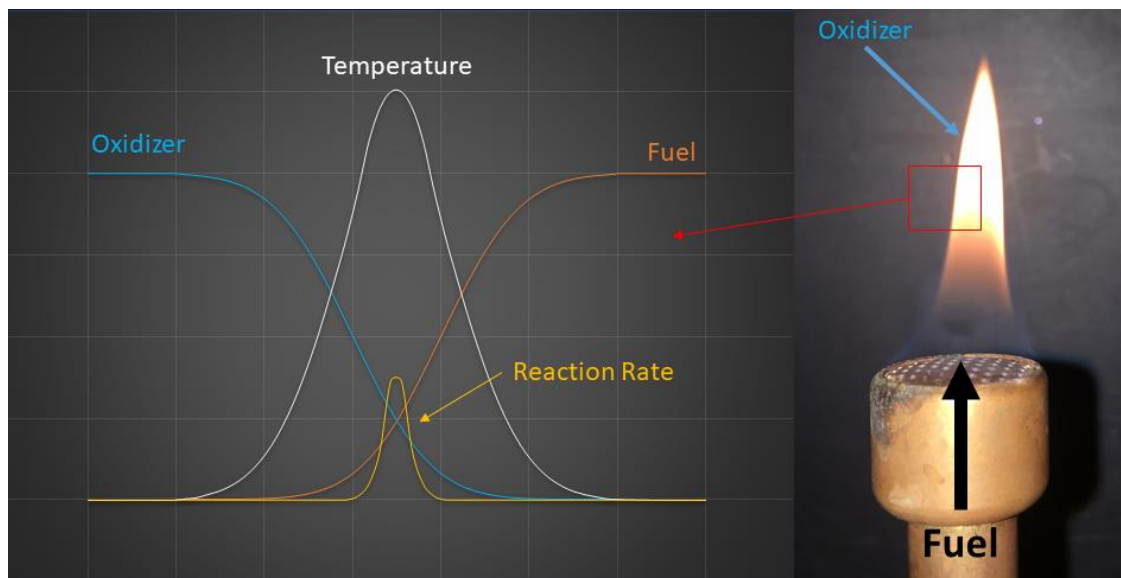
Figure 7. An example of a non-premixed flame/diffusion flame with fuel and oxidizer concentration, temperature, and reaction rate profiles.
