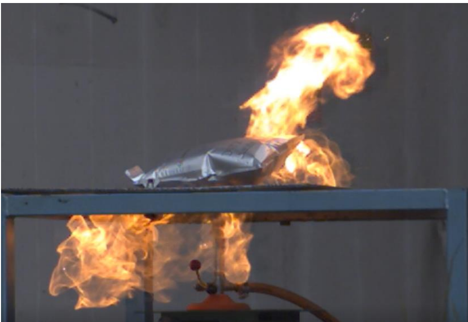
Figure 5. A photo of a pouch cell externally heated by a bunsen burner
