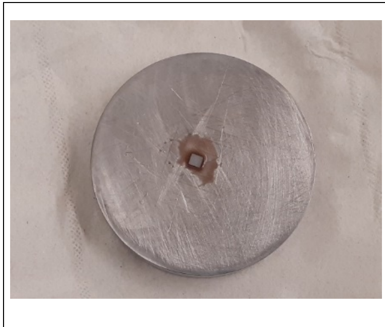
Figure 17. Shows the resistor chip fixed on polishing fixture using mounting paste wax.
