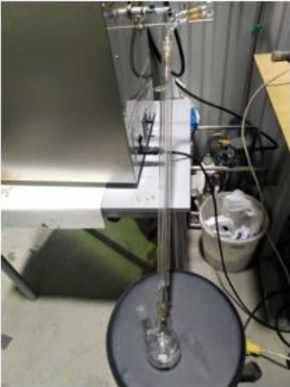
Figure 3.4 Experimental setup carried out in the USN laboratories. Starting from the top left and proceeding clockwise, it is shown: 1. reactor inserted in the furnace with closed flange, 2. reactor inserted in the furnace with open flange, 3. aluminum capsule acting as reactor and 4. water-cooled condenser.
