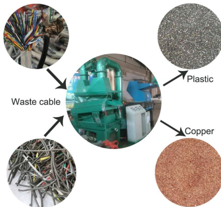
Figure 1.1 Metals and plastic separation in cable processing [3]
