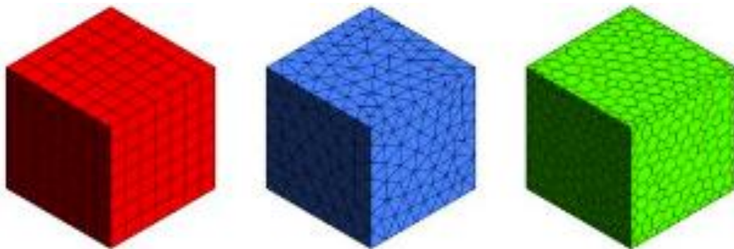
Figure 5.1: Basic cell types for CFD. Left is hexahedral, the middle is tetrahedral, and right is polyhedral cells [43]
