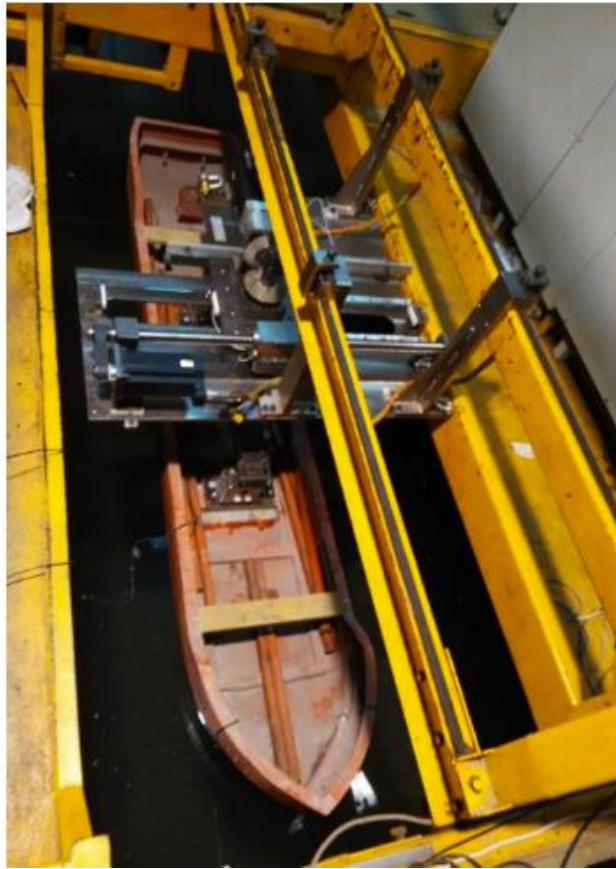
Figure 2.6: Tow tank test setup for a ship [16]
