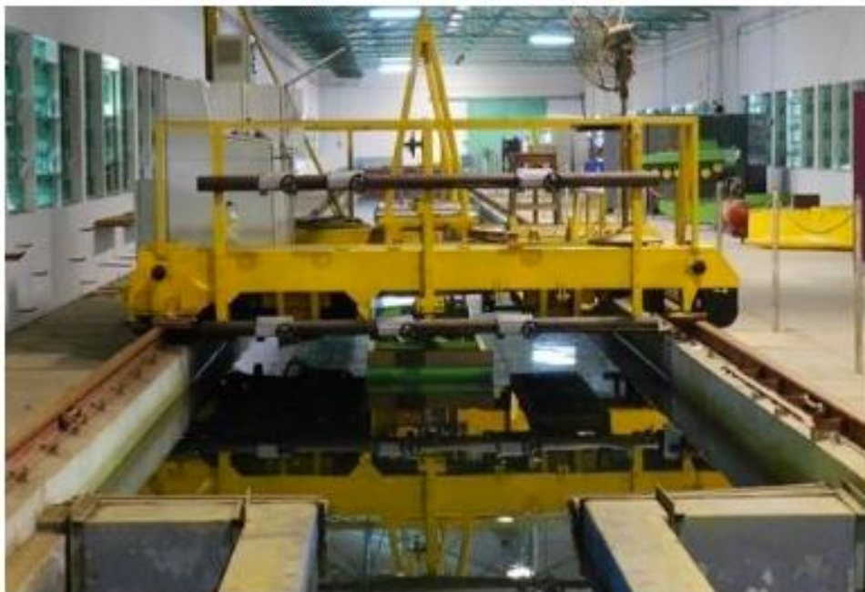
Figure 2.5: Illustration of a tow tank with test carriage [16]
