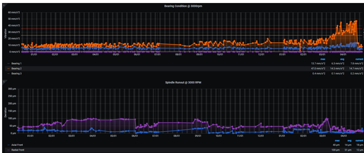
Figure 3.8: Source vibration data (upper part of the graph) and runout for the axial and radial front (lower part) with a duration of about 15 months.
