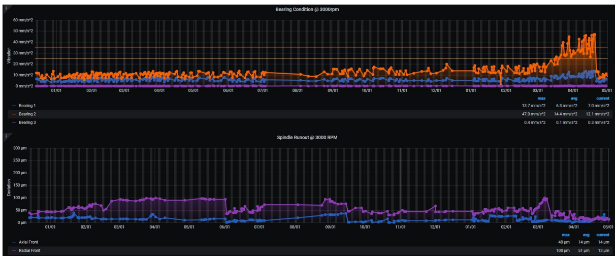
Figure 1.2: Screenshot of source data of vibration, measured in mm/s^2 (top graph), and runout (bottom graph) data, measured in \mu m from Copilot.
