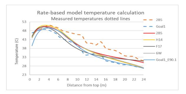
Figure 4-10: Calculated temperatures for the test cases with rate-based model. Measured temperatures with dotted lines for comparison. (CO<sub>2</sub> removal equals test results for all calculations)
