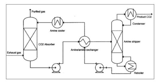
Figure 2-1: Principles for  $CO_2$  removal process based on absorption in amine solution ( $\emptyset i \ 2012$ )
