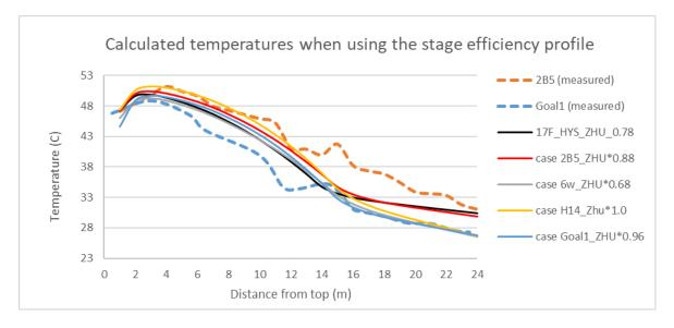
Figure 4-5: Calculated temperatures with the profiled stage efficiencies. Measured values included with dotted lines for comparison. ( $CO_2$  removal equals test results for all calculations)
