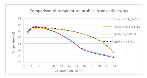
Figure 4-4: Comparing H-14 temperature calculations with earlier work
