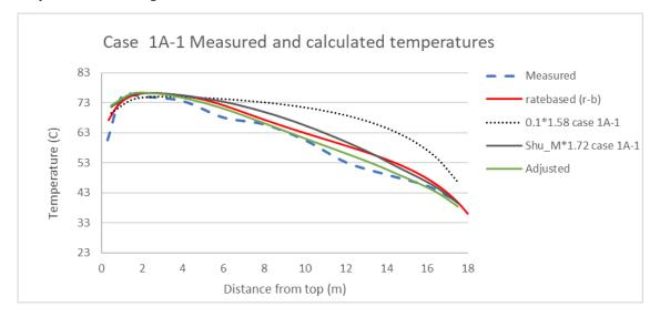
*Figure 5-4: Calculated and measured temperatures for 1A-1 test case. (CO<sub>2</sub> removal equals test results for all calculations)*
