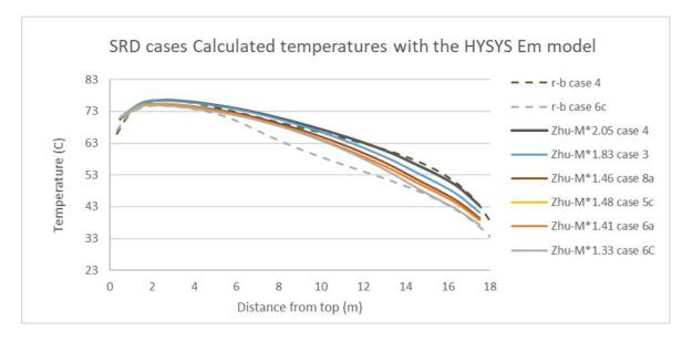
Figure 5-3: Calculated temperatures for the SRD test cases with the Aspen HYSYS Em model using the Zhu-M profile as a basis. The rate-based model calculations for cases 4 and 6c included for comparison. (CO<sub>2</sub> removal equals test results for all calculations)
