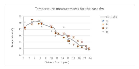
Figure 4-1: Measured and average absorber temperatures for case 6w
