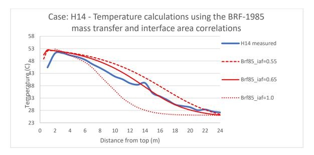
*Figure 4-11: Measured and calculated temperatures for the case H14 and sensitivity to correlations and interface area factor (Fagerheim 2019)*
