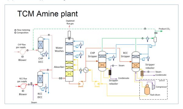
Figure 2-2: TCM amine plant with main items and fluid flows (Hamborg, et al. 2015)
