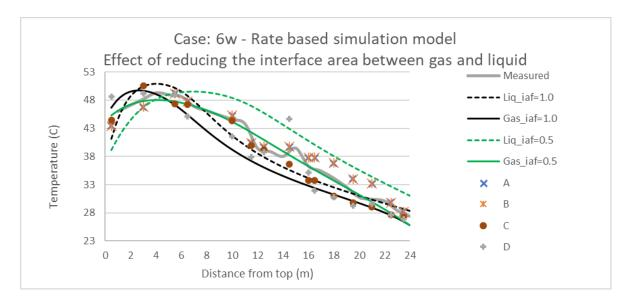
Figure 4-9: Measured and calculated temperatures for the case 6w with rate-based model
