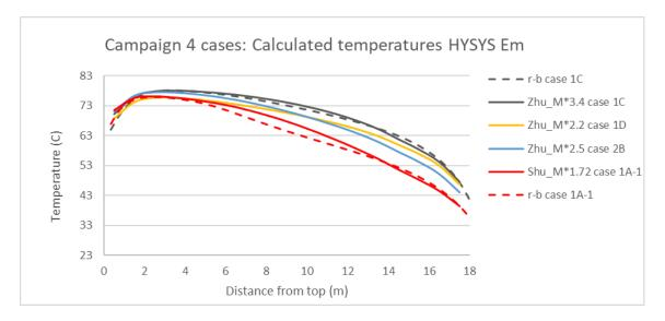
Figure 5-6: Calculated temperatures for the selected Campaign 4 test cases with the Aspen HYSYS Em model using the Zhu-M profile as a basis. The rate-based model calculations for cases 1C and 1A-1 are included for comparison. (CO<sub>2</sub> removal equals test results for all calculations)
