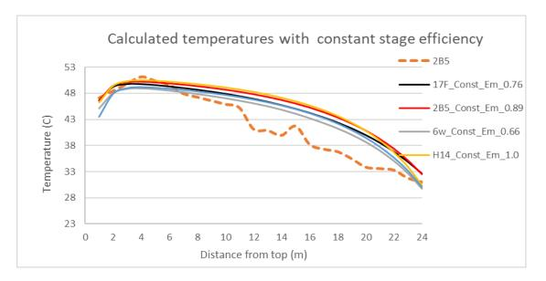
Figure 4-6: Calculated temperatures with constant stage efficiencies. Measured value included with dotted lines for comparison. (CO<sub>2</sub> removal equals test results for all calculations)
