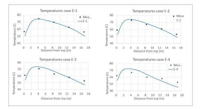
Figure 5-7: Calculated temperatures compared with measurements for the Esbjerg cases. (Liquid holdup factor 0.72 for all calculations)
