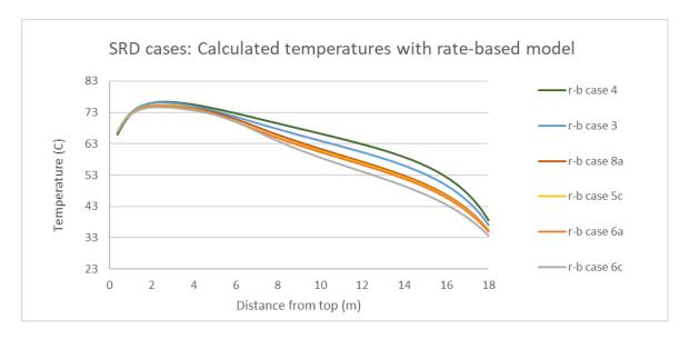
*Figure 5-2: Calculated temperatures for SRD cases with the rate-based model. (CO<sub>2</sub> removal equals test results for all calculations)*
