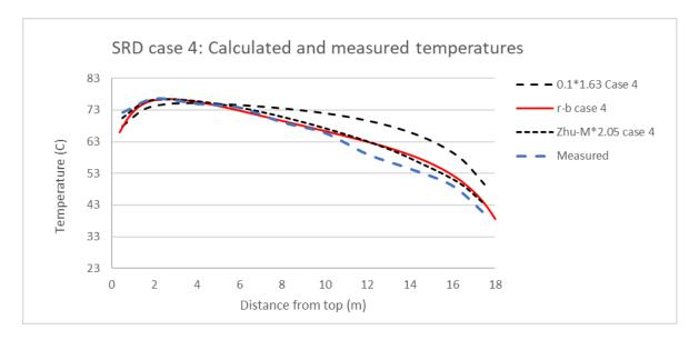
*Figure* 5\_1: *Calculated and measured temperatures for SRD case* 4. (*CO*<sub>2</sub> *removal equals test results for all calculations*)
