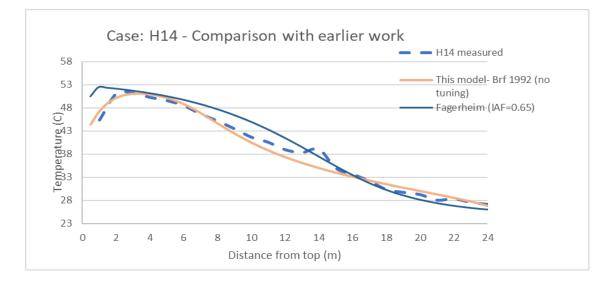
Figure 4-7: Comparison of case H14 temperature calculations with earlier work and with measured temperatures
