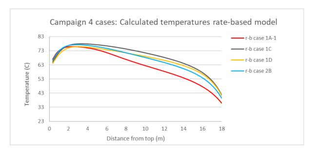
*Figure 5-5: Calculated temperatures for SRD cases with the rate-based model. (CO<sub>2</sub> removal equals test results for all calculations)*
