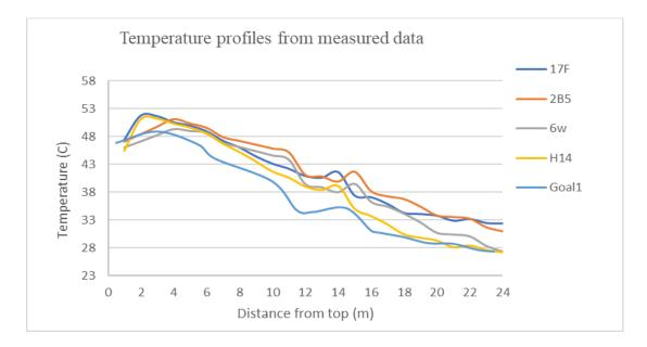
Figure 4-2: Absorber temperature profiles based on the test case measurements
