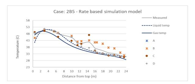
*Figure 4-8: Measured and calculated temperatures for the case 2B5 with rate-based model*
