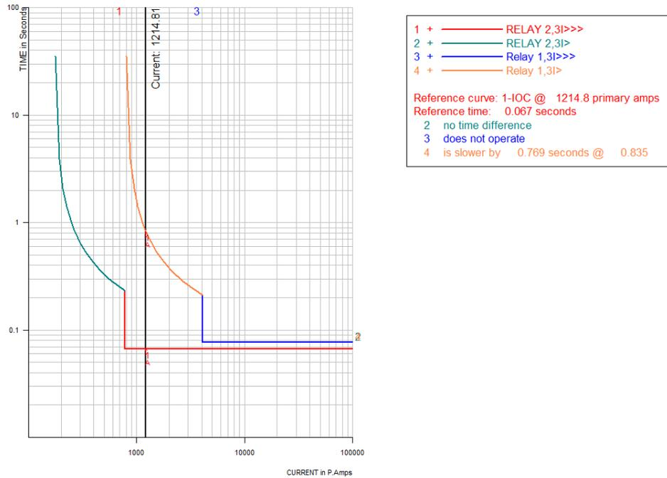
Figure 3-4 Relay Characteristics for 3 Phase Fault, Bus 6.
