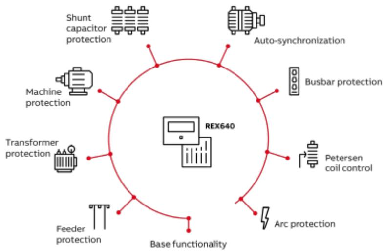
Figure 2-2 REX640 Protection Functions
