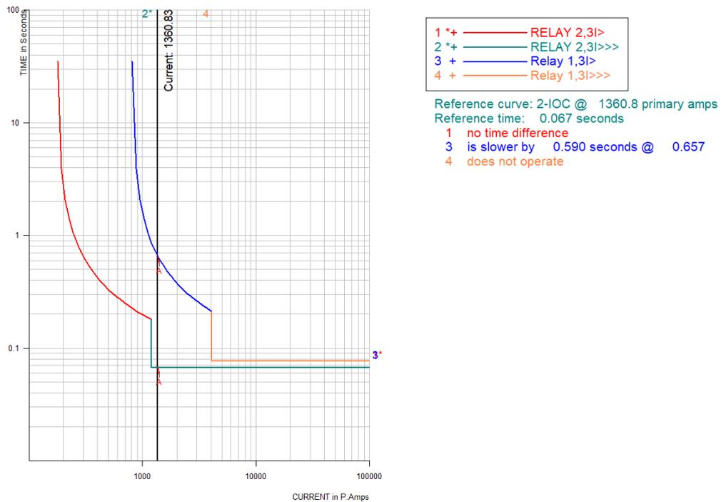
Figure 3-7 Relay Characteristics for L-L Fault at Bus 2
