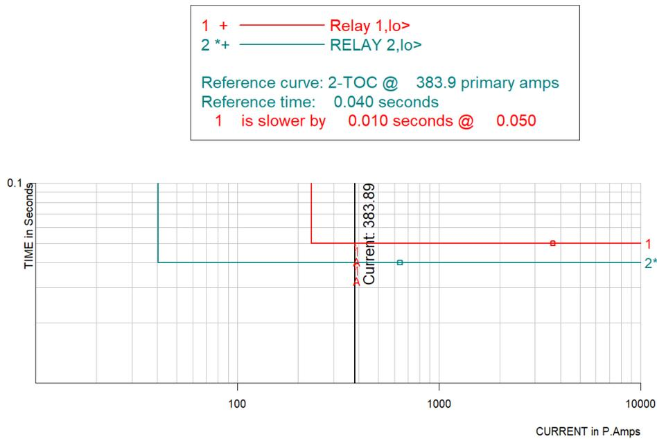
Figure 3-8 Line to Ground Fault at Busbar 6
