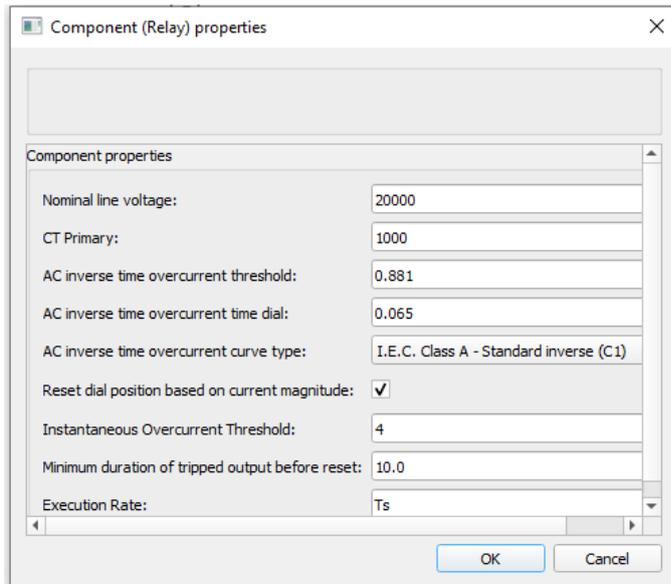
Figure 4-4 Relay R1 Setting in Typhoon HIL
