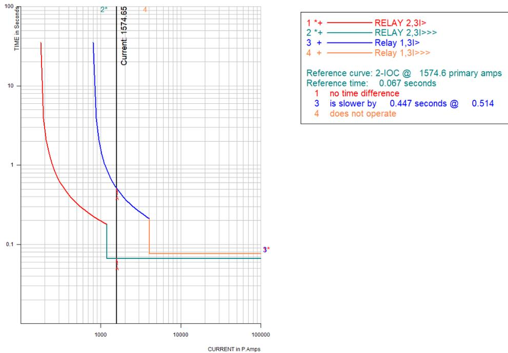
Figure 3-5 Relay Characteristics for 3 Phase Fault, bus 2.
