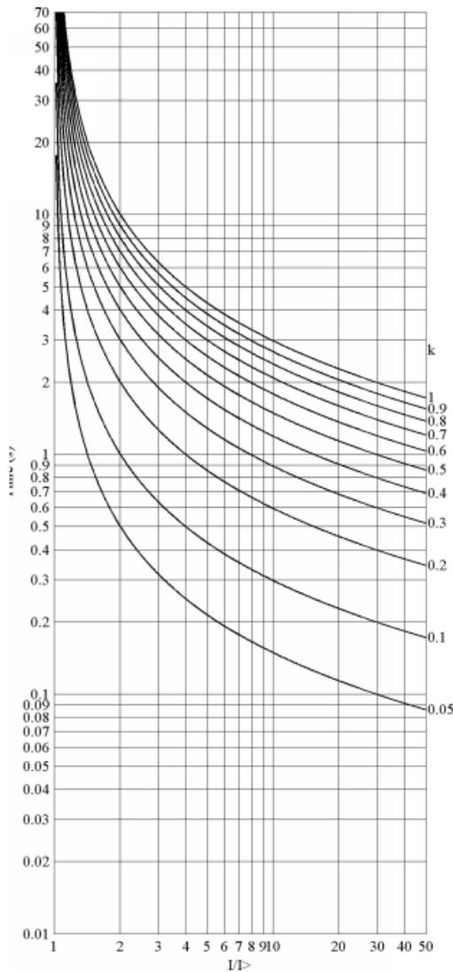
Figure 3-3 IEC Normal Inverse Curve, REF615
