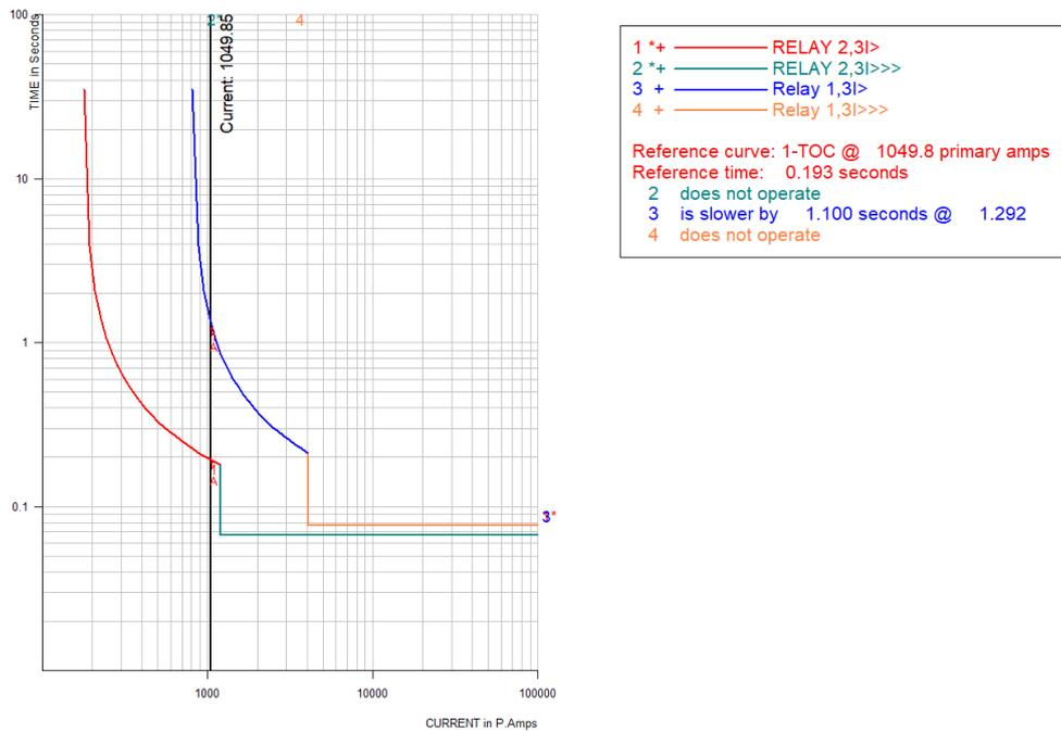
Figure 3-6 Relay Characteristics for L-L Fault at Bus 6
