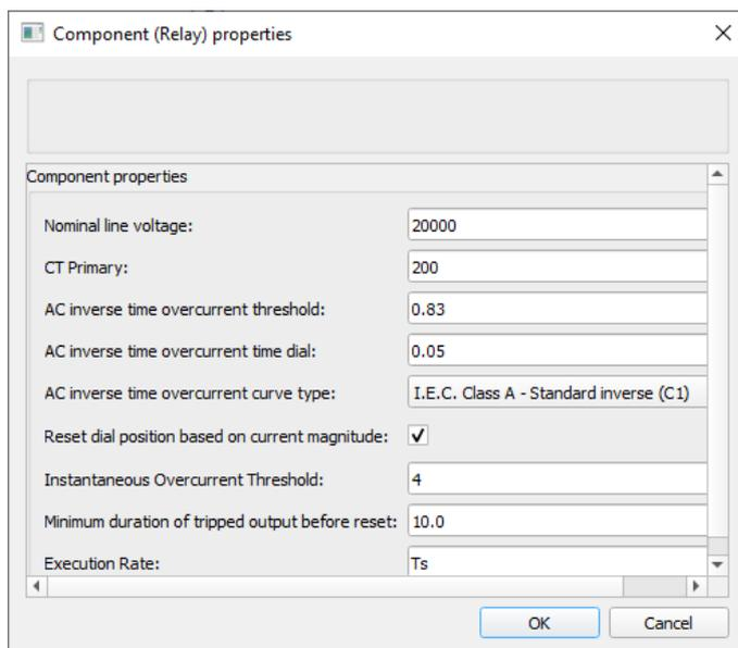
Figure 4-5 Relay R2 Setting in Typhoon HIL
