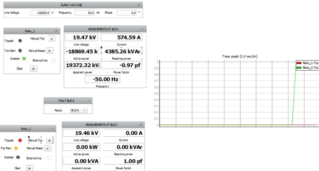
Figure 4-7 Tripped Relay
