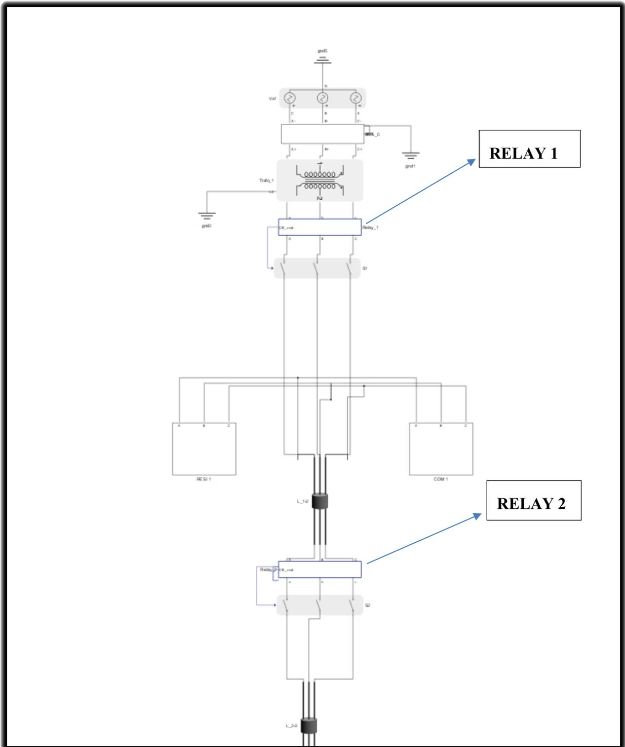
Figure 4-2. CIGRE Network Model in Typhoon HIL
