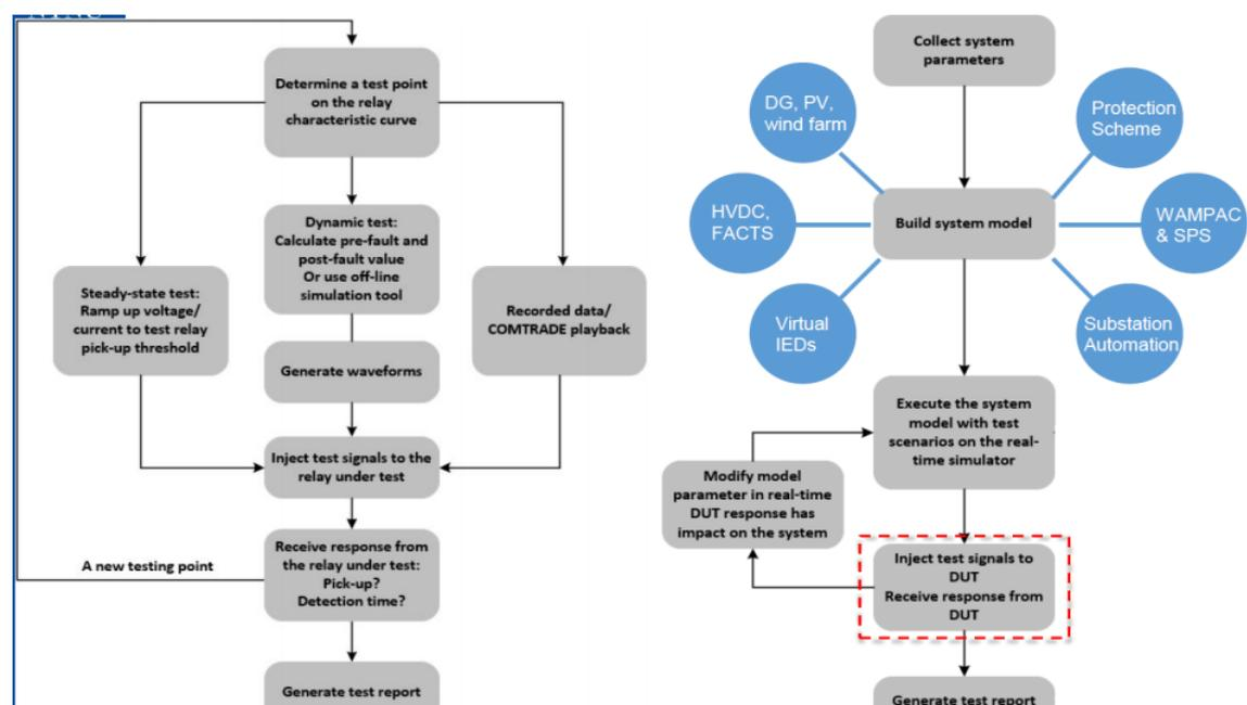
Figure 1-1. Traditional Testing Versus HIL Testing
