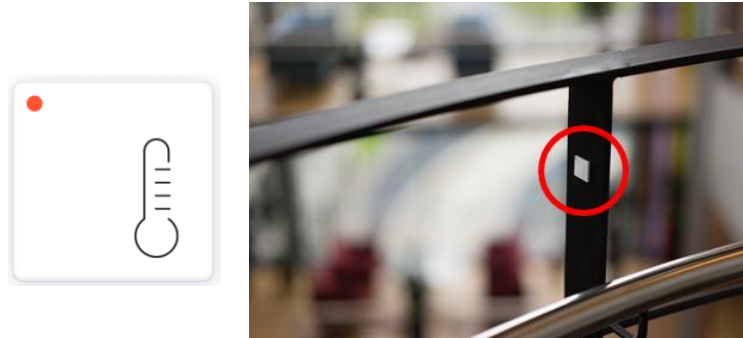
Figure 3.4: The Wireless Temperature Sensor from Disruptive Technologies where the right picture shows an example of sensor placement. [50]
