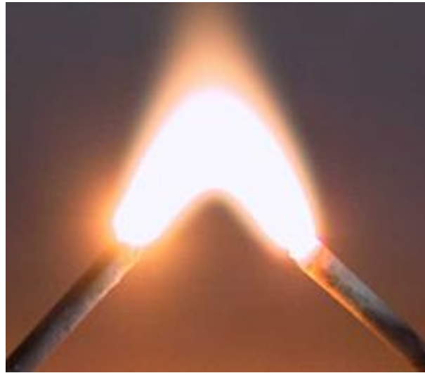
Figure 2.1: An electric arc formed in the gas gap between two electrodes [3]
