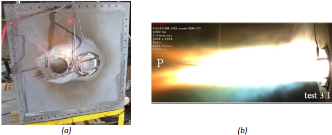
Figure 3.5: (a) bursting disc (b) pressure and hot gases released through the pressure relief openings [15]
