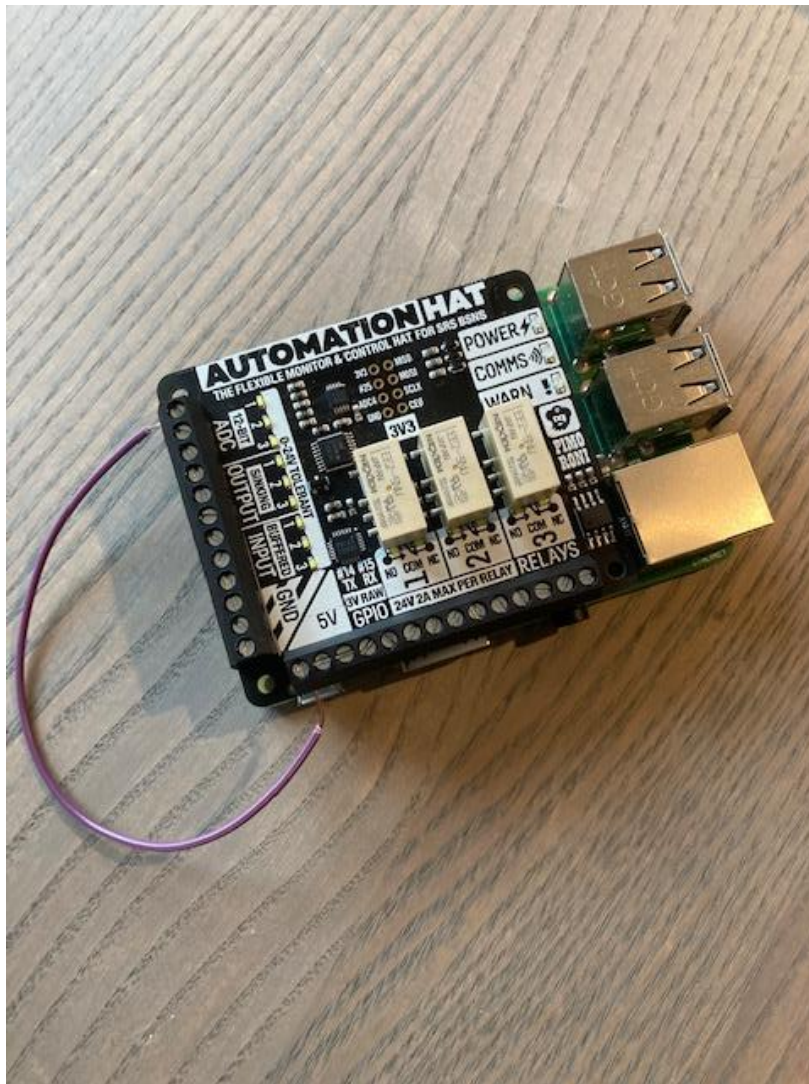
Figure 3.55: A wire connected between the analog input channel and 5 V channel on the Automation HAT board
