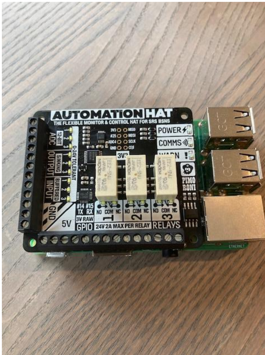
Figure 3.54: The Automation HAT board attached to the Raspberry Pi Model B+ board
