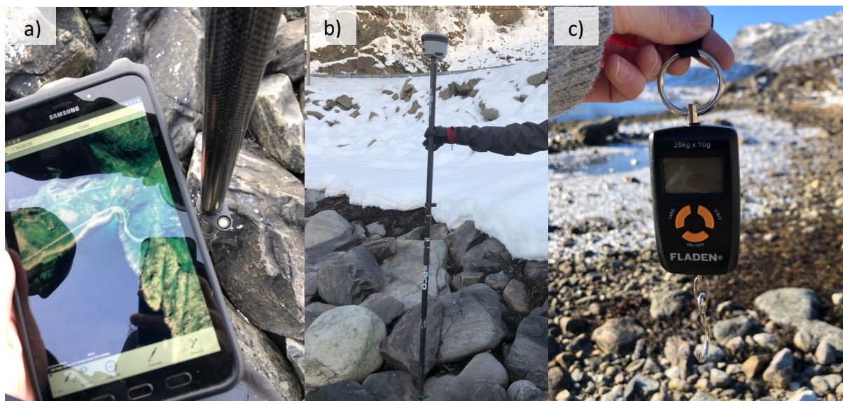
Figure 7. Equipment used during field surveys at the three beaches. a) the tablet using the Software Trimble Penmap, b) Trimble R2 GPS unit, and c) fishing weight used for weighing litter. Photo: Vilde S. Solbakken.
