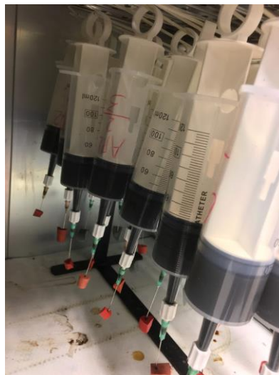
Figure 3.2 Medical plastic syringes with inoculum and APL inside the incubator.
