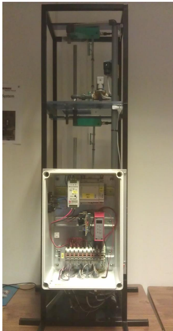
Figure 3-1: The serial two tank model setup.
