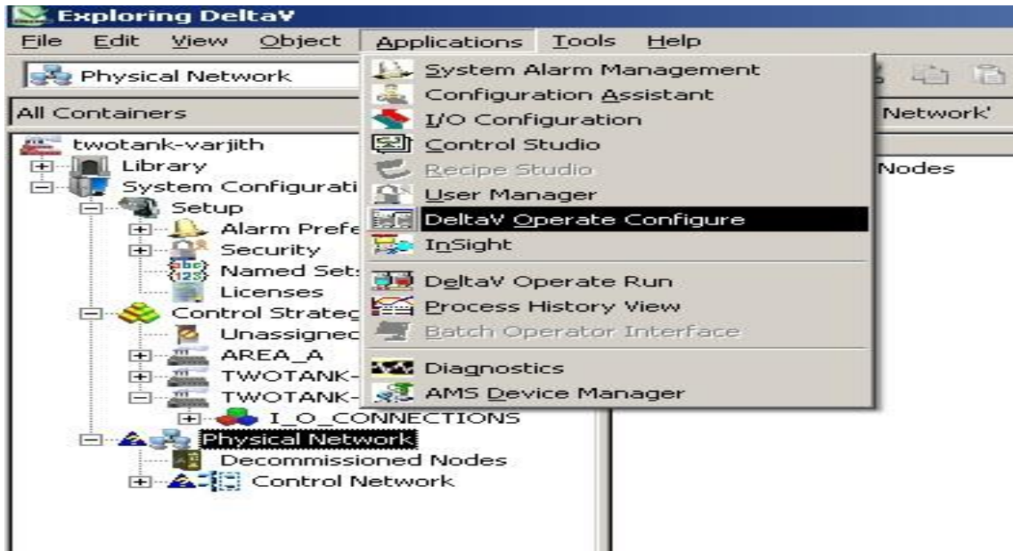
Figure 4-13: shows the path of DeltaV operate configure panel in the DeltaV Explorer.
