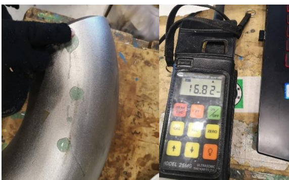
Figure 2. Measuring of 270 on plane 1 [left] and reading from NPS 6 SCH 80 Bend 1 [right]
