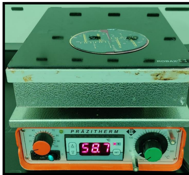
Figure 25:Soft Baking for enhancing PDMS and Au bonding.
