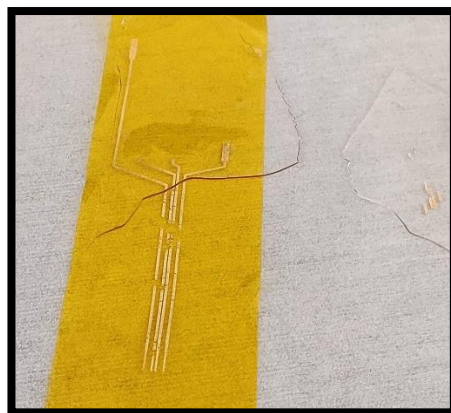
Figure 45: Failed Adhesion test for 300nm Electrode.
