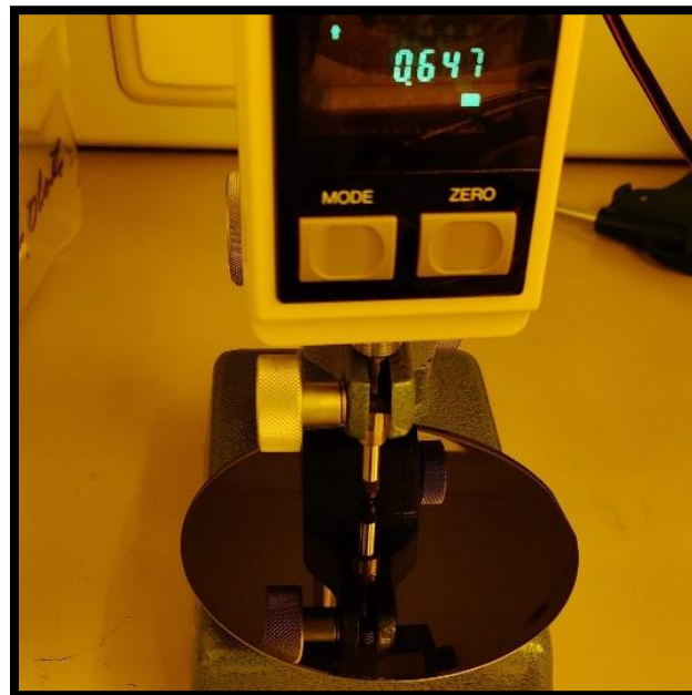
Figure 29: Measurement of PDMS thickness.
