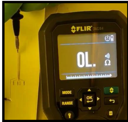
Figure 44: Non-Conductive Part of 300nm Electrode
