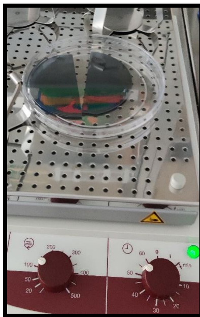
Figure 23: PDMS deposited wafer immersed in MPTMS on chemical shaker.
