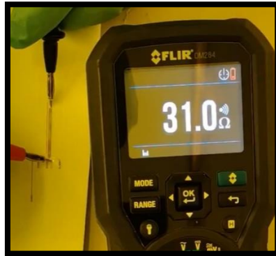
Figure 43: Conductive Part of 300nm Au Electrode.
