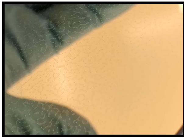
Figure 39: Bubble structure on Au thin film.
