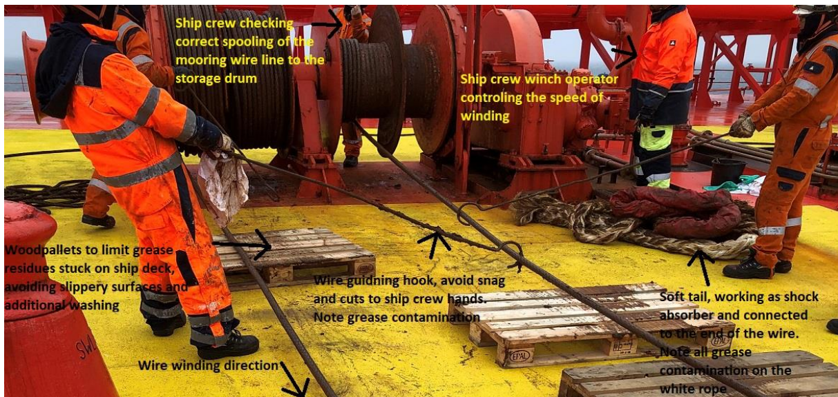
Figure 4. Ship crew performing maintenance of forward breast winch and mooring line.
