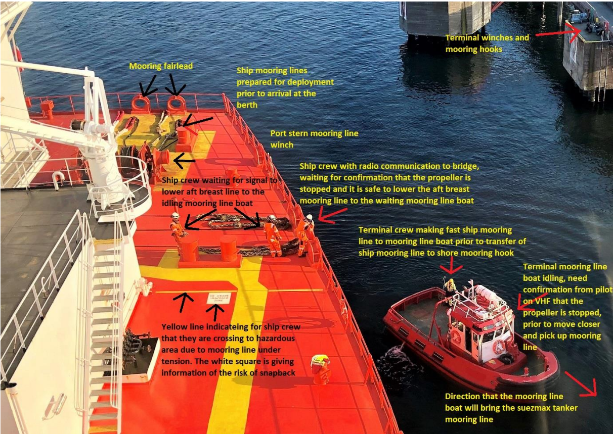
Figure 5. Ship crew stationed at the poop deck area performing mooring operation together with the terminal crew.
