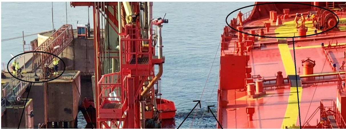
Figure 6b. Detailed view of forward mooring process.
