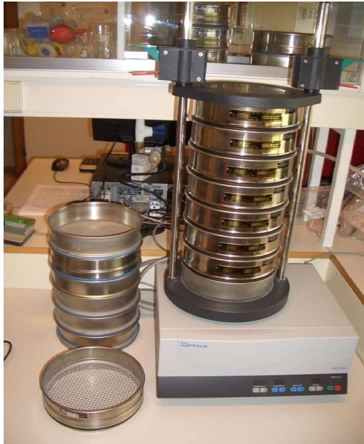
Figure 4.5: The vibratory sieve-column with different size of sieves.
